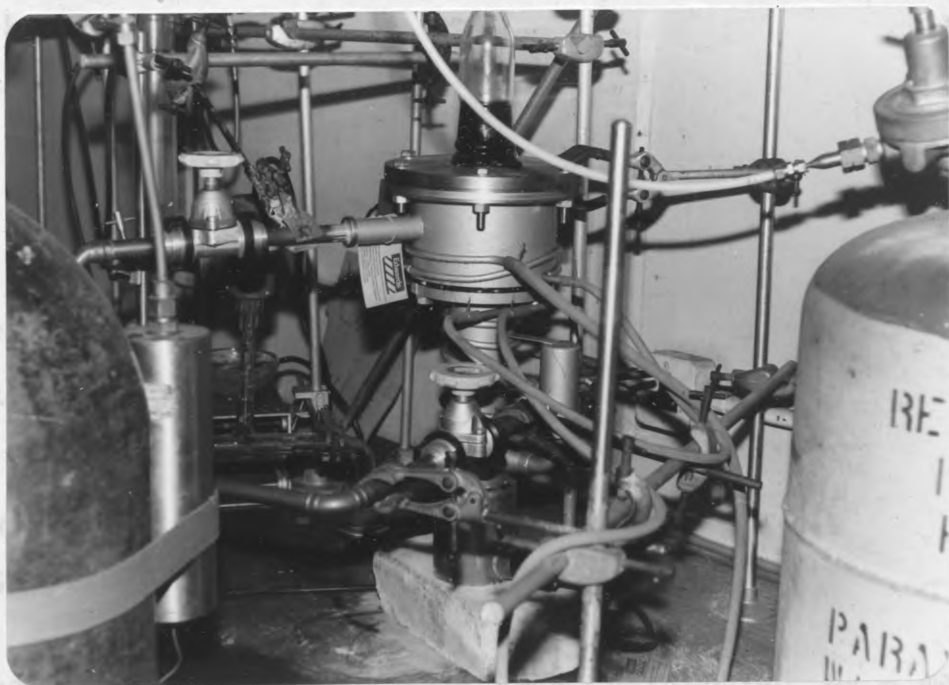
Plate 6 Diffusion pump showing muff-coupled valves
