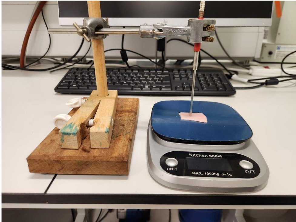
Figure 7.1: Diffuse reflectance experiment setup of Porcine Skin measurement
