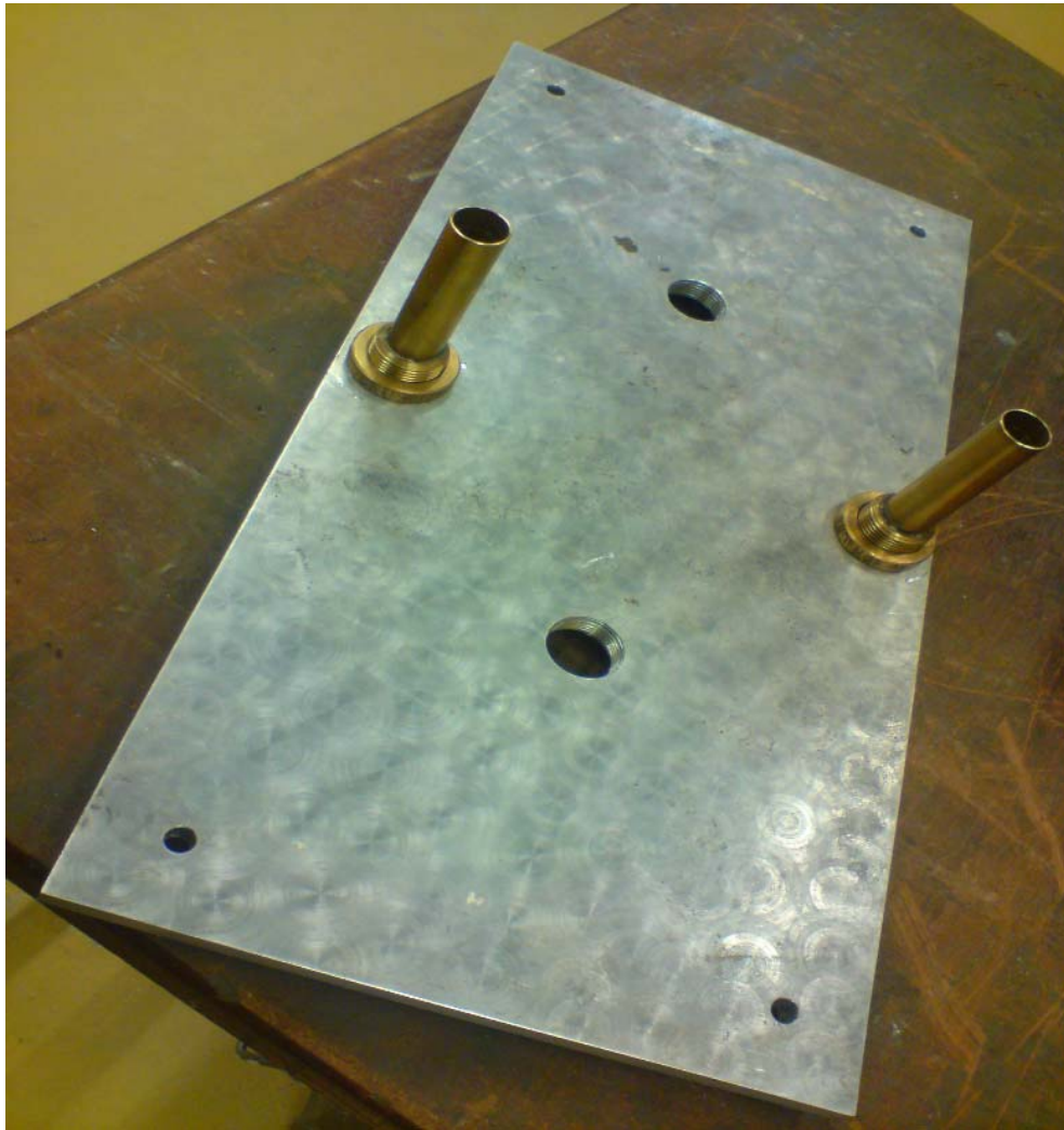
Figure 4.10 Photograph of guide apparatus for the pile cutter
