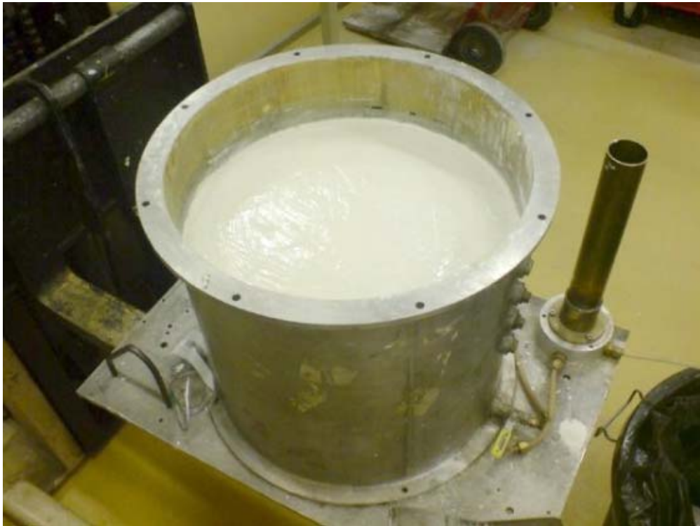
Figure 4.3 Stainless Steel Tub in which the soil sample is prepared and the model piles are constructed
