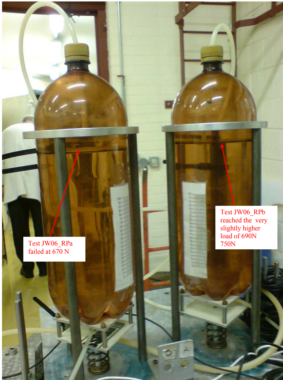
Figure 6.44 Photograph showing water levels in bottle reservoirs after test JW06
