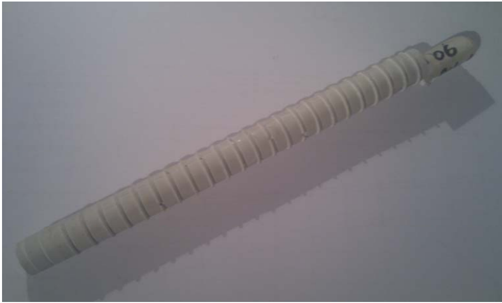
Figure 7.5 Photograph of model pile from test JW06_RPa
