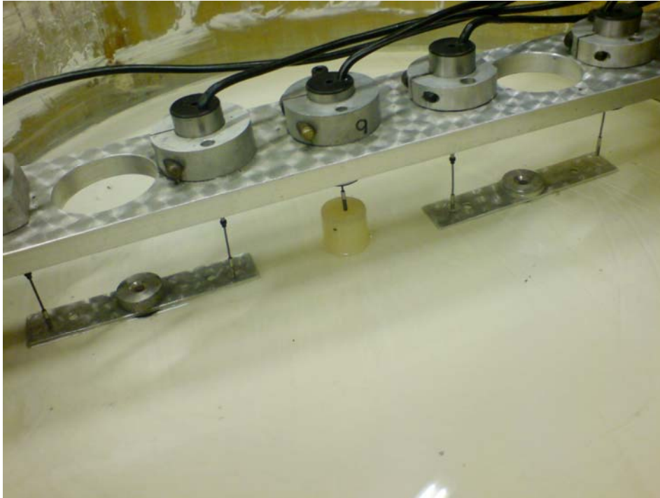
Figure 6.9 Photograph showing loading apparatus on removal from centrifuge after test JW01 – water level gives indication of load applied
