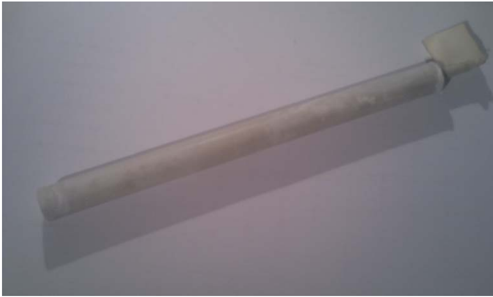
Figure 7.2 Photograph of model pile from test JW01_SP
