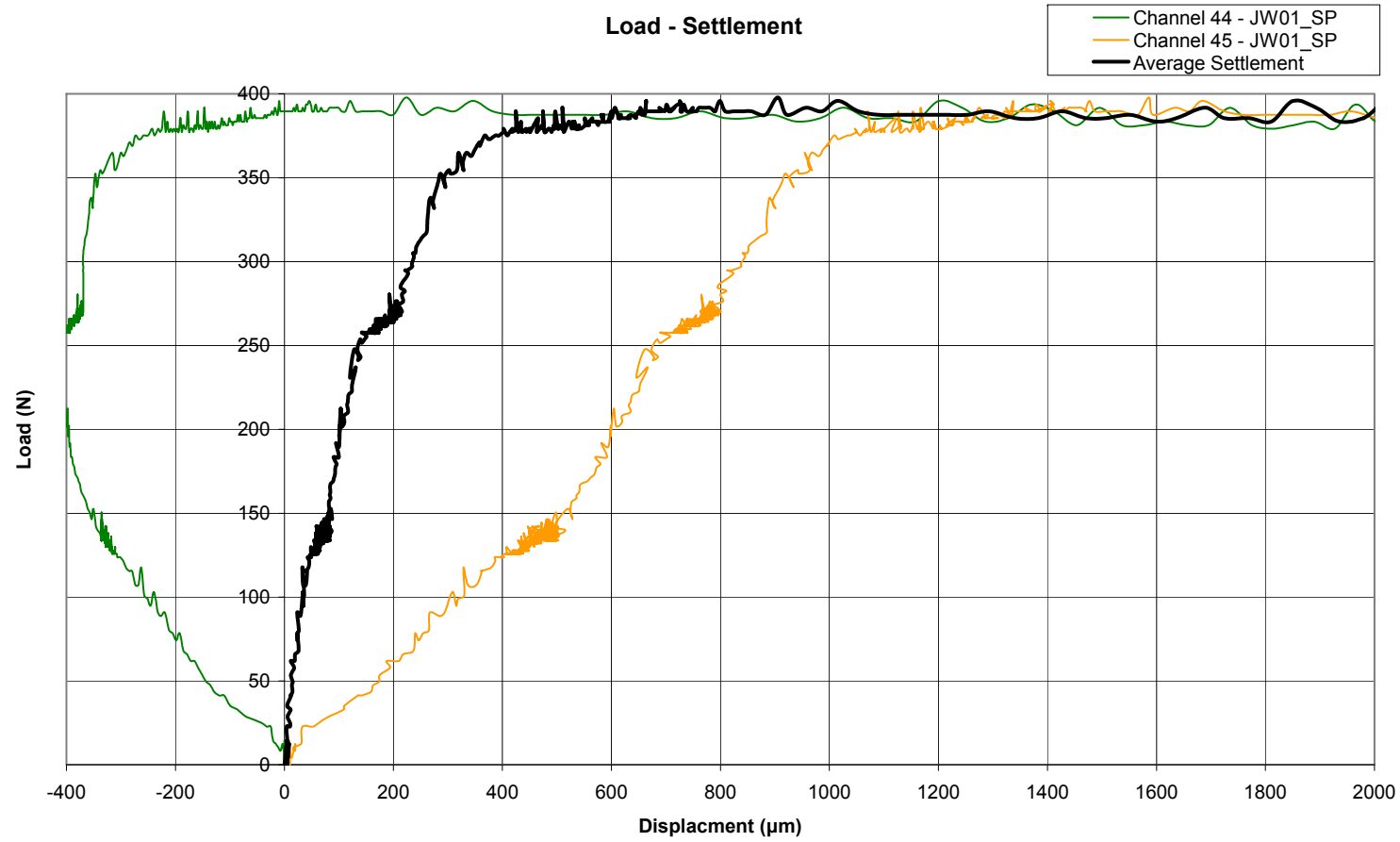
Figure 6.5 Test JW01_SP: Load-Settlement Graph
