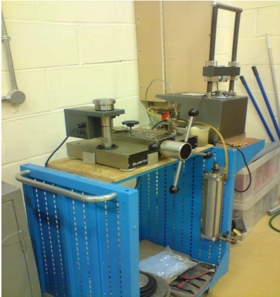
Figure 5.3 Photograph of the Budenberg for calibration of the load cells
