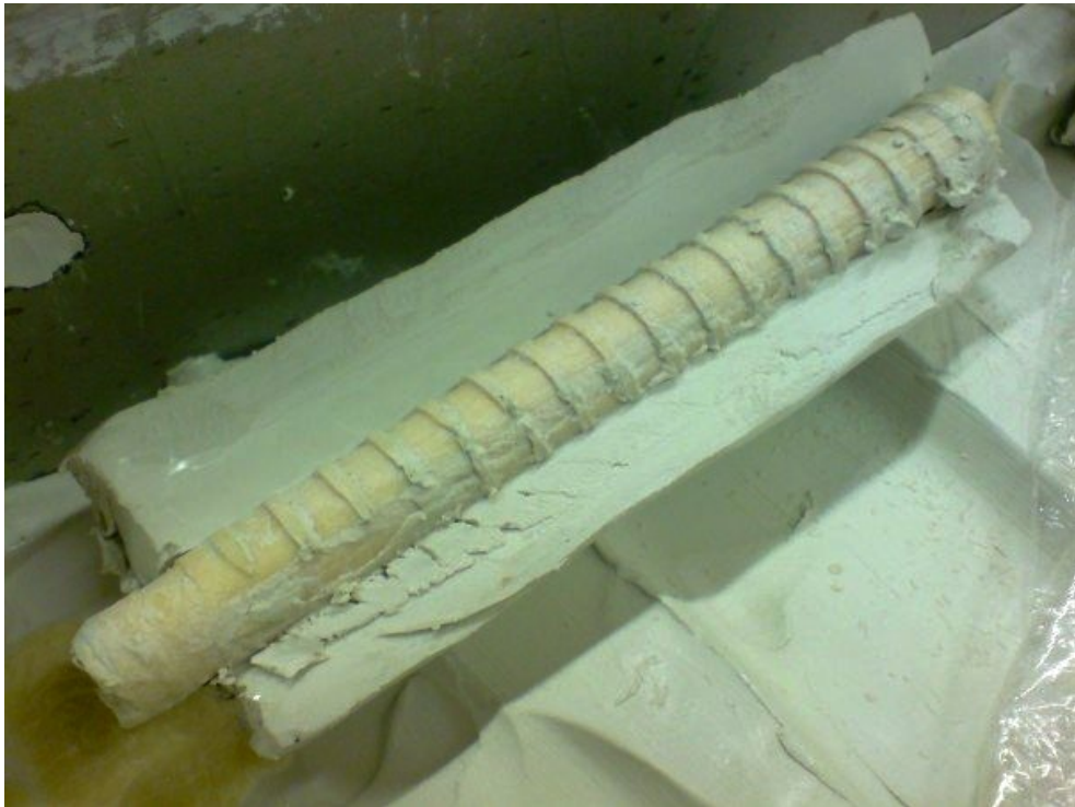
4.9 Photograph showing resin pile formed by first test of rib cutting mechanism
