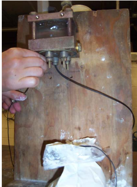
Figure 5.1 Calibration chamber for PPT calibration
