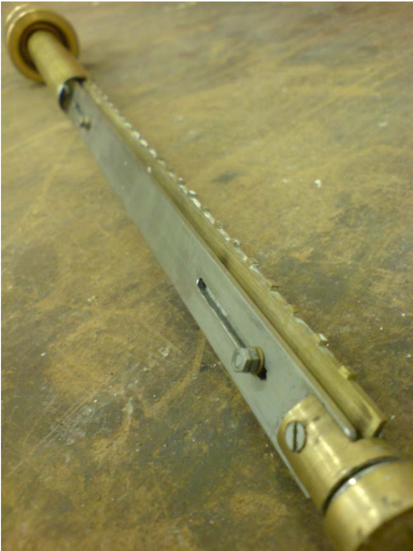
Figure 4.8 Photograph of complete rib-cutting tool
