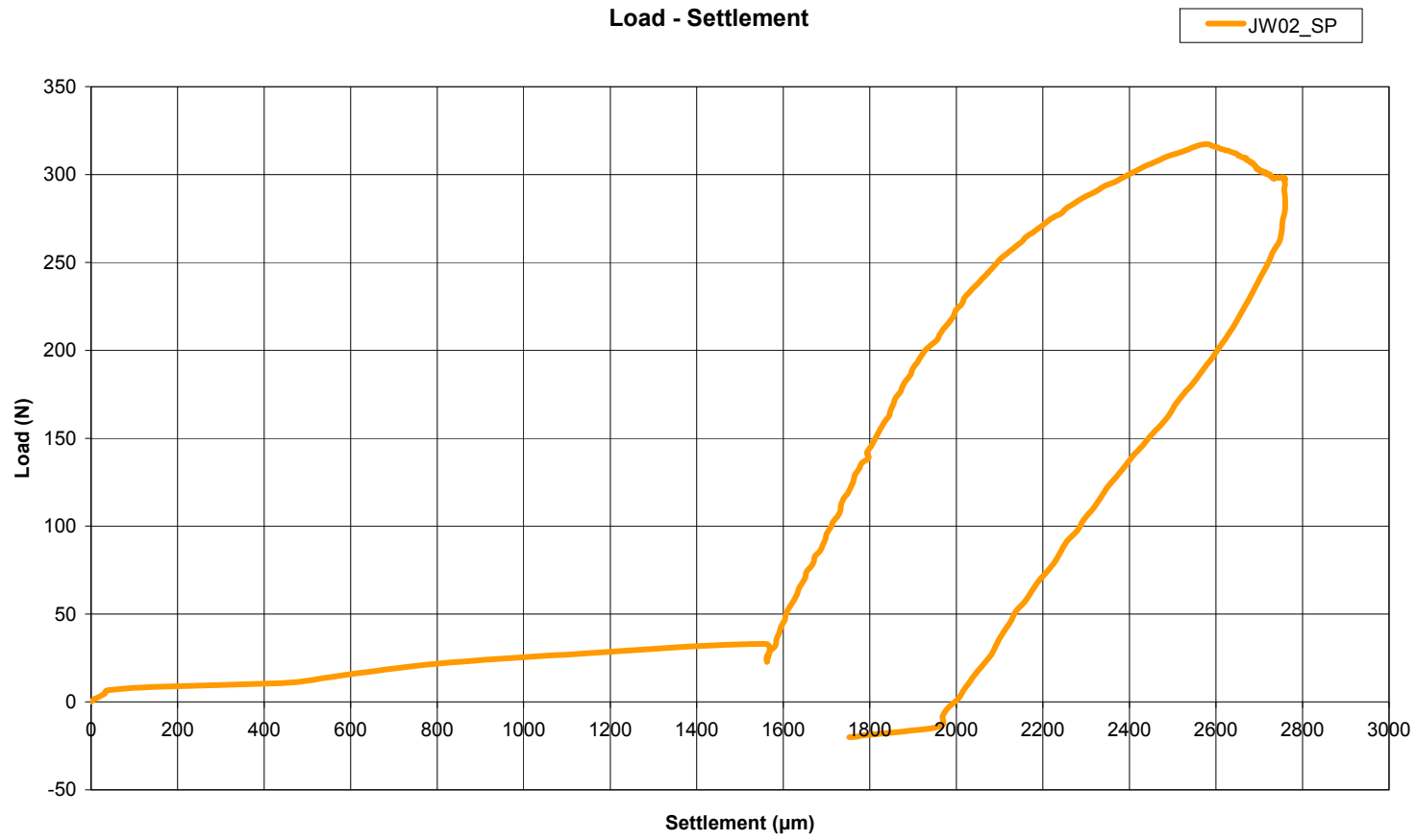
Figure 6.14 Test JW02: Load-Settlement Graph
