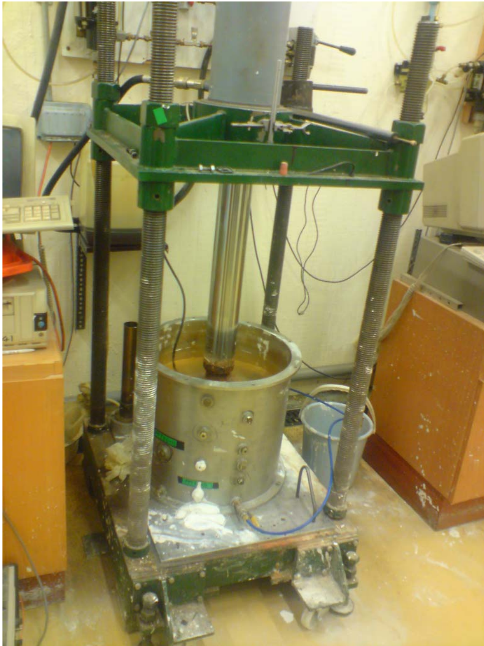
Figure 4.4 Photograph of a soil sample being prepared in the consolidation press
