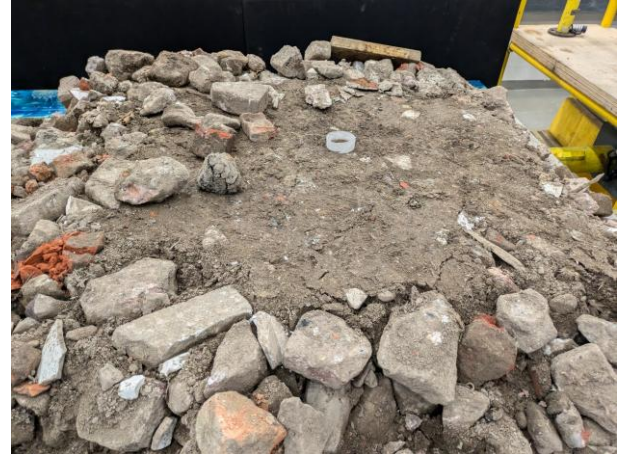
Figure 4. Sample of recycled 6F5 aggregate following a test.
