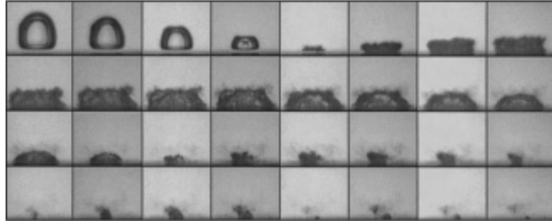
(a) Collapse evolution of a bubble near a solid surface.
