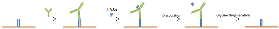
Figure 4-6: A conventional SPR strategy to measure affinity of FcRn to an antibody. A CM5 chip (orange) with immobilised anti-Fab fragment (blue) is used to capture the bNAb (green). The analyte hFcRn (blue) is flowed over the chip, followed by a wash with the running buffer (dissociation). The captured antibody is removed from the chip using glycine (regeneration)
