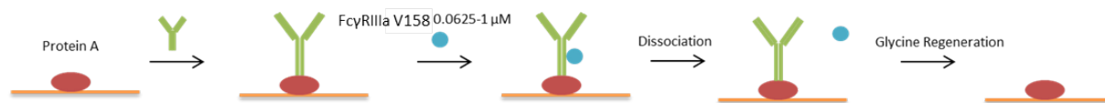
Figure 4-1: Strategy for determining binding kinetics of Fc \gamma RIIIa V158 to bNABs using SPR. A CM5 chip (orange) with immobilised protein A (red) was used to capture the respective bNAB (green). Fc \gamma RIIIa V158 (blue) was flowed over the chip in various concentrations, followed by a wash with running buffer (dissociation). To remove the captured bNAB, glycine was flowed over the chip (regeneration step)
