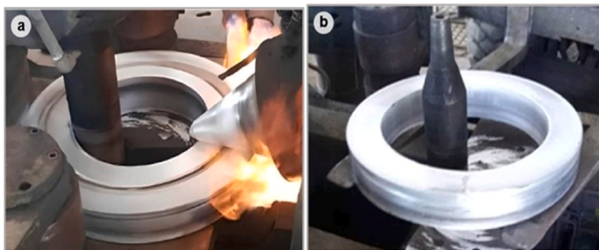
Fig. 8. a) Deformation in ring rolled alloy b) SPD proceed alloy [109].
