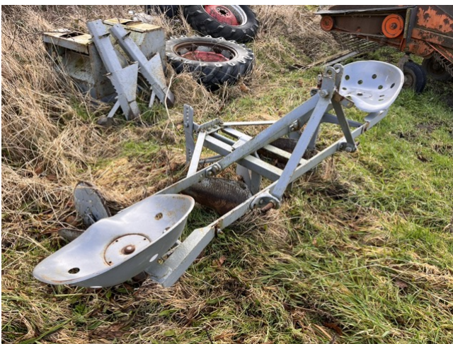
Figure 3: Potato planter. Attached to a tractor, it creates three furrows in the soil, while two workers sitting on the seats drop potatoes in.
