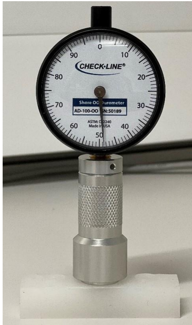
Figure 25: Measuring the hardness of silicone tissue using a Shore-00 Durometer. Measurements were taken from multiple locations on the tissue and averaged [152].
