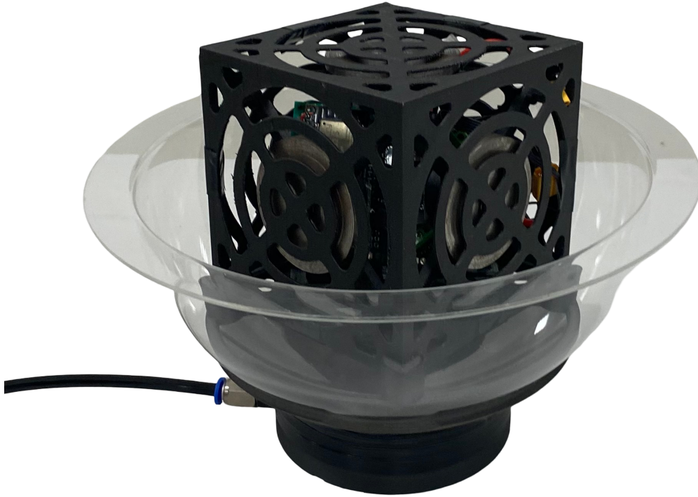
Figure 5.24: Assembled air bearing platform with CubeSat mounted.
