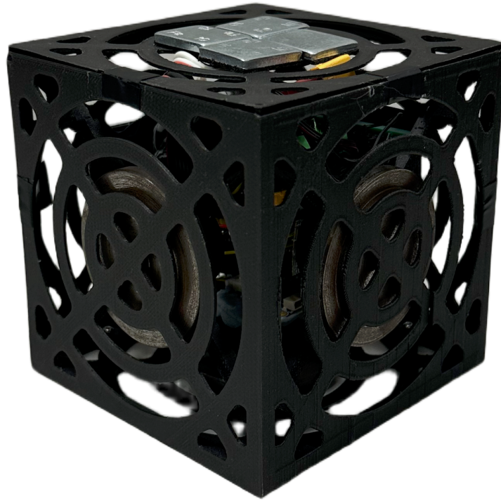
Figure 5.21: Final assembly of the 1U CubeSat hardware platform.
