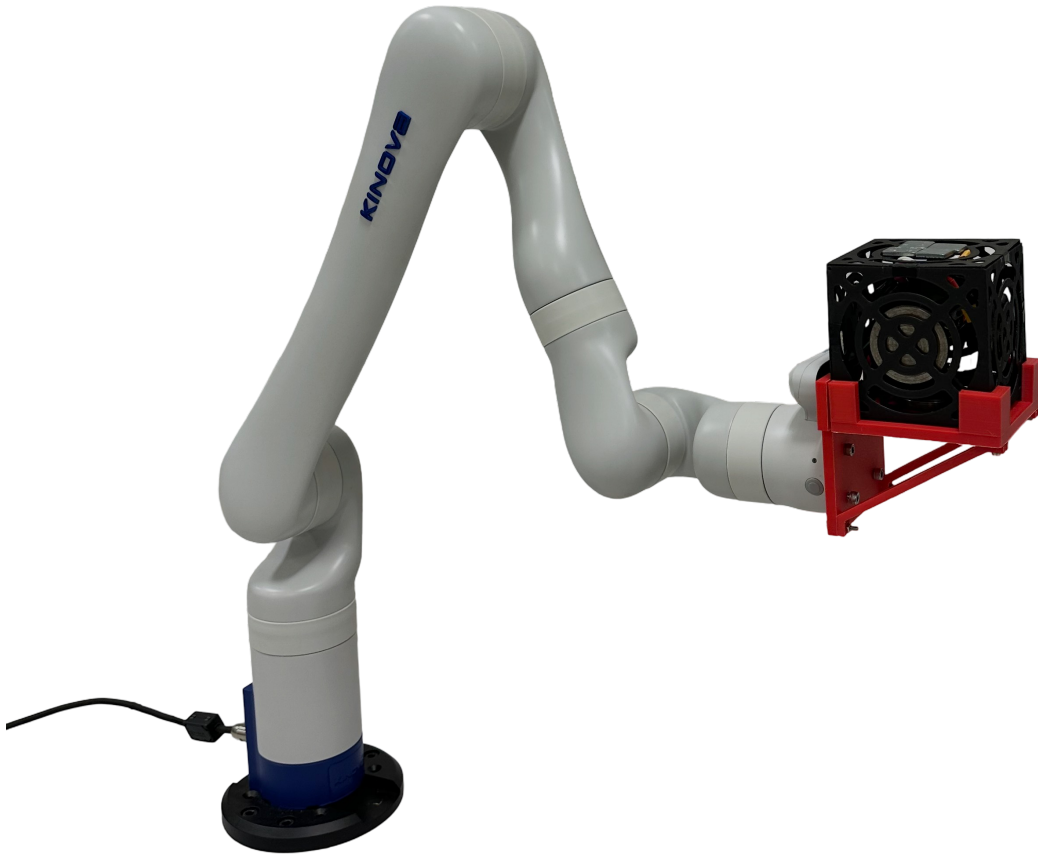
Figure 5.25: Rendezvous testing platform with mock CubeSat mounted.
