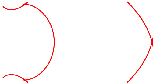
Figure 6.16: Examples of undercuts that occur on the inner rotor profiles of a sinusoidal rack generated profile for non-valid regions in Figure 6.14 (a).
