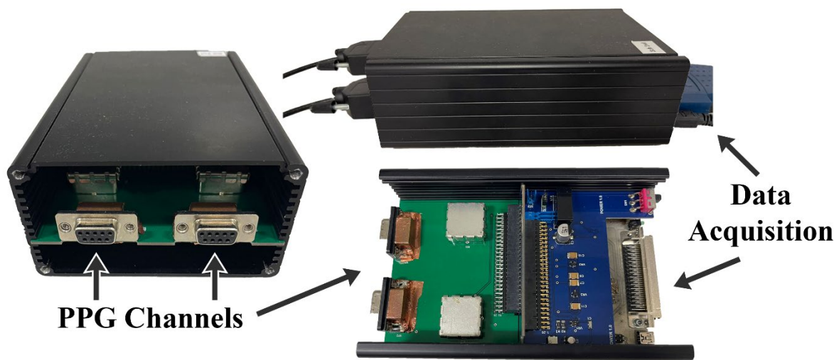
FIGURE 5-13. The outside and inside structure of the ZenPPG. Used for dual-channel PPG signal acquisition and processing.
