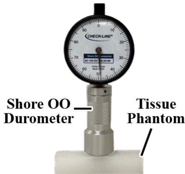
FIGURE 6-4. Shore hardness measurement of silicone tissue using a Shore OO durometer. The device is positioned vertically with its flat base in contact with the sample surface to ensure consistent readings. This method quantifies tissue stiffness, with lower values indicating softer materials suitable for mimicking compliant biological tissue.
