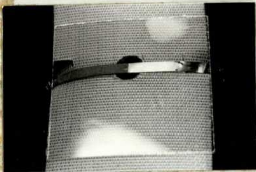
PLATE 3 FOIL THERMOCOUPLE PLACED ON ADHESIVE SIDE OF PERMACEL TAPE WITH MICA SHEET ON TOP. THE DARKER HALF OF THE FOIL WAS THE SILVER PLATED ONE.
