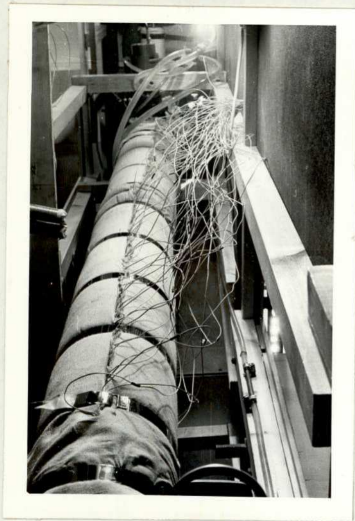
Plate 11. View inside test section and pre-heater enclosure upwards towards the test section exit.
