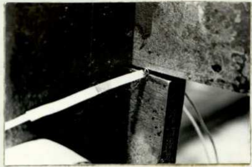
PLATE 2 CRIMPING THE THERMOCOUPLE WIRE TO THE END TAG.
