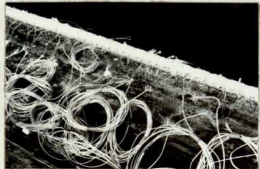
PLATE 8 VIEW OF INSULATED THERMOCOUPLES ON A PORTION OF THE TEST SECTION.
