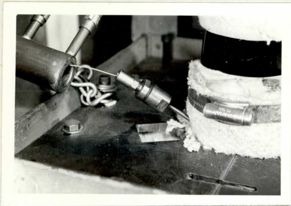
Plate 13. View of thermocouple gland cooler removed to show sealing gland for sheathed thermocouples.
