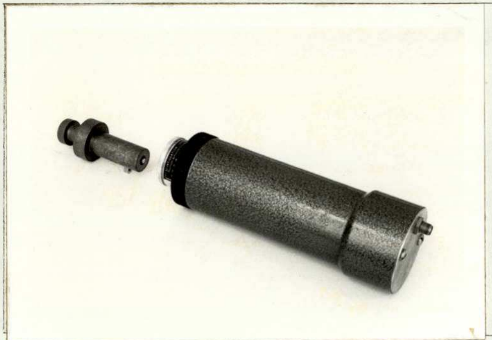
PLATE 26 Source holder showing radioisotope pellet and sodium iodide crystal - photomultiplier tube.
