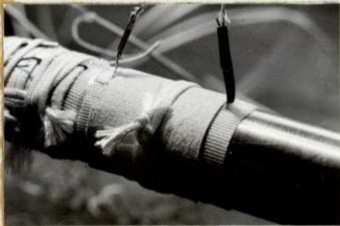
PLATE 5 ASBESTOS PAPER WRAPPED AROUND TUBE AND SECURED WITH VIDAFLEX GLASS FIBRE STRING.
