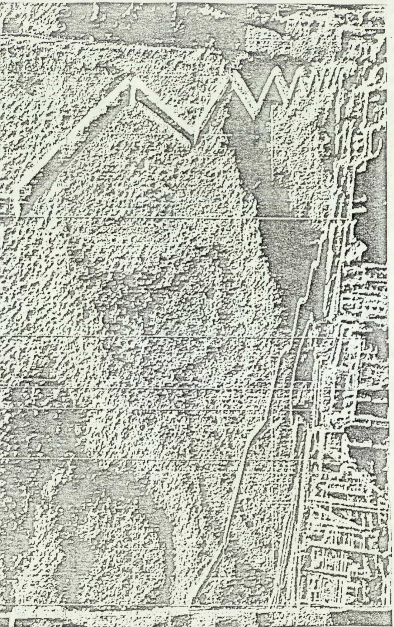
Fig. 6.30 Direction map using four masks to obtain the 8 compass direction (the direction measure is codified as light intensity in the image).
