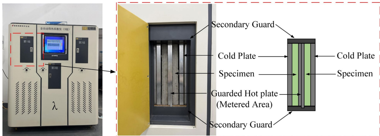
Fig. 7 Experimental device for thermal conductivity
