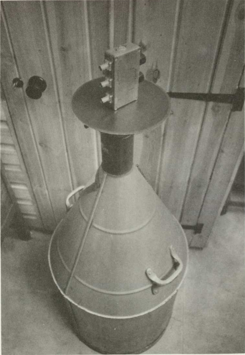
Plate 3. Bridge and junction probe inserted into liquid helium dewar
