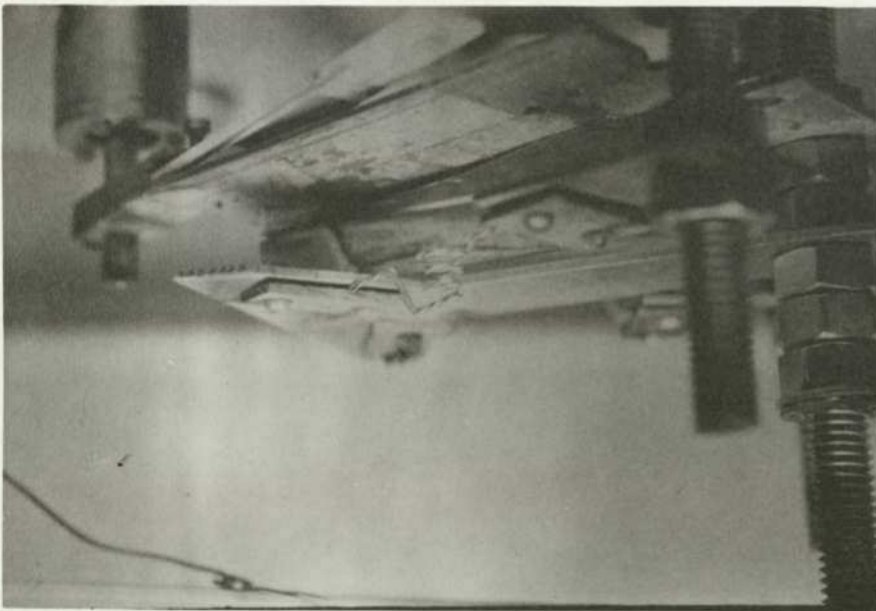
Plate 2b. Tungsten basket and masks for aluminium evaporation
