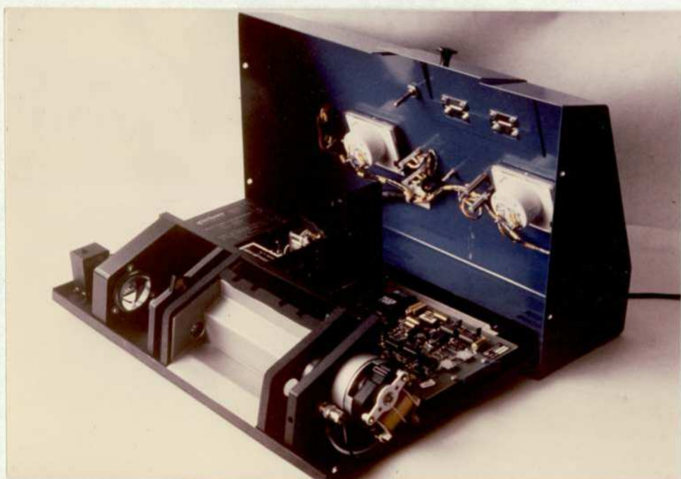
Fig. 5.7 The interior of the Refined Oil Colorimeter.
