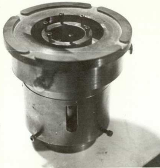
Plate 6.4.1. The grinding jig and adaptor used in fabricating the transducers for the acousto-optic devices.
