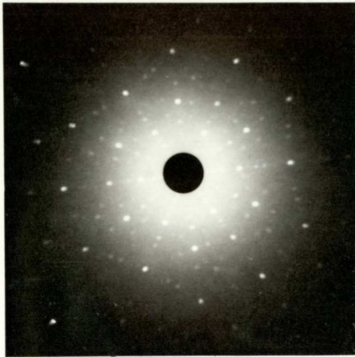
Plate 5.6.1. X-ray laue pattern for \text{LiNbO}_3 along the crystallographic z axis.
