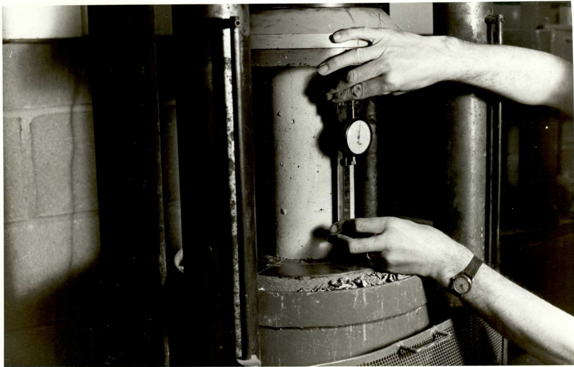
PLATE: 11 Micro-Concrete Cylinder under compression test.
