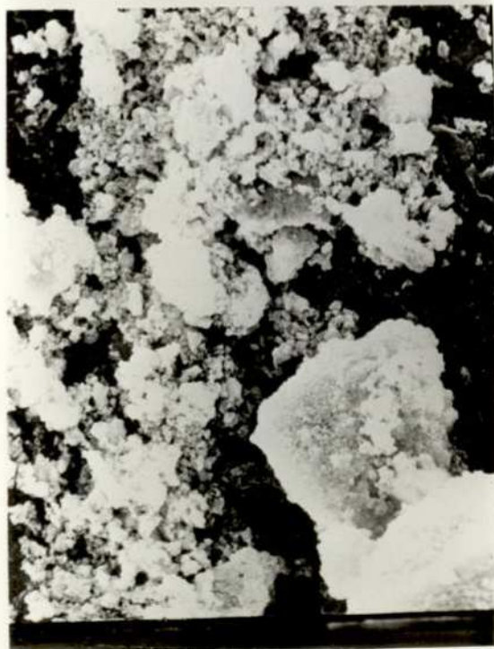
(c). Cobalt-nickel sulphide prepared at 550°C for 12 hrs.
