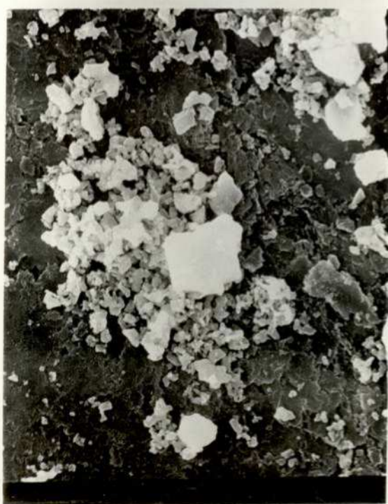
(b). Cobalt-nickel sulphide prepared at 400°C for 12 hrs.
