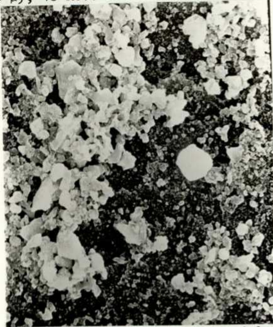
(a) Thermal decomposed cobalt-nickel oxide.
