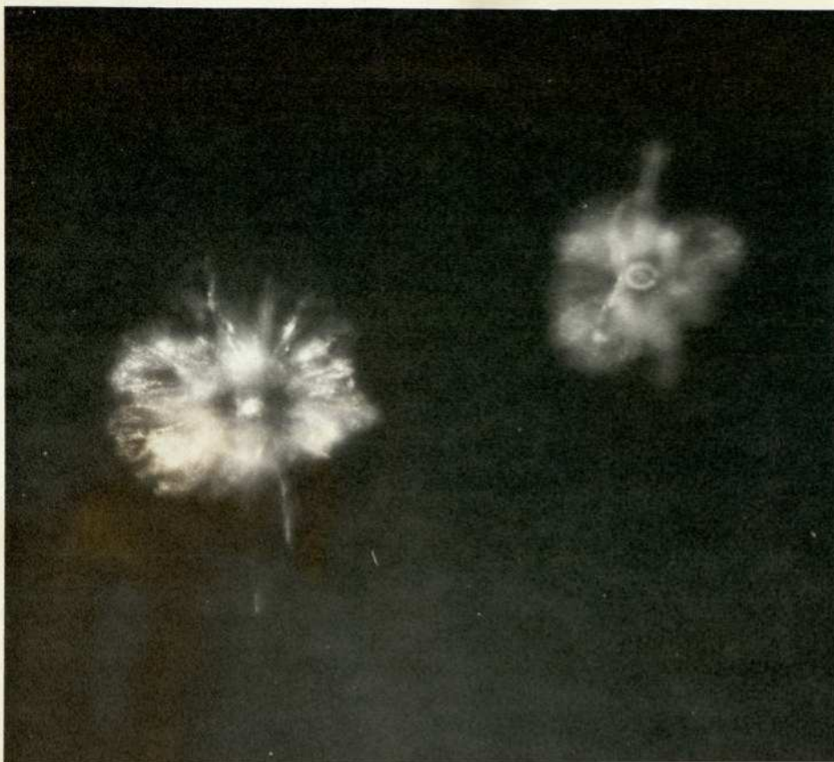
Inclusion Damage in ADP
