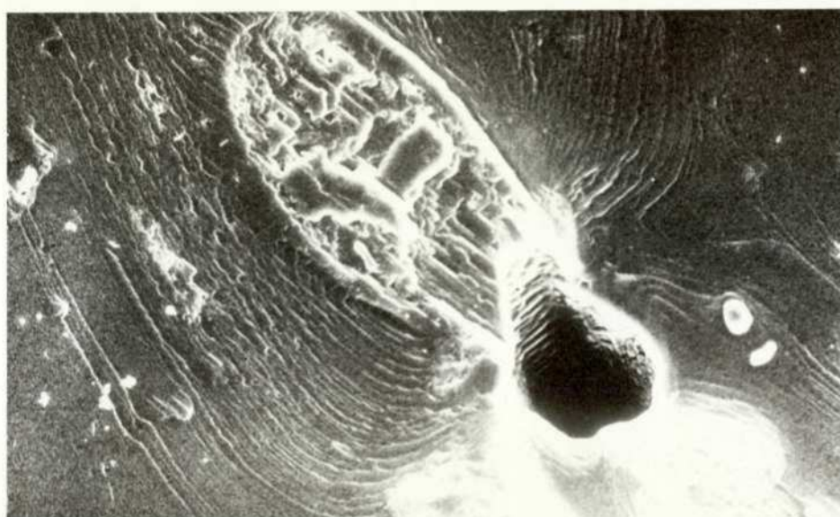
Fig 6.9(b) Large Void Fractured ( \times 300 )
