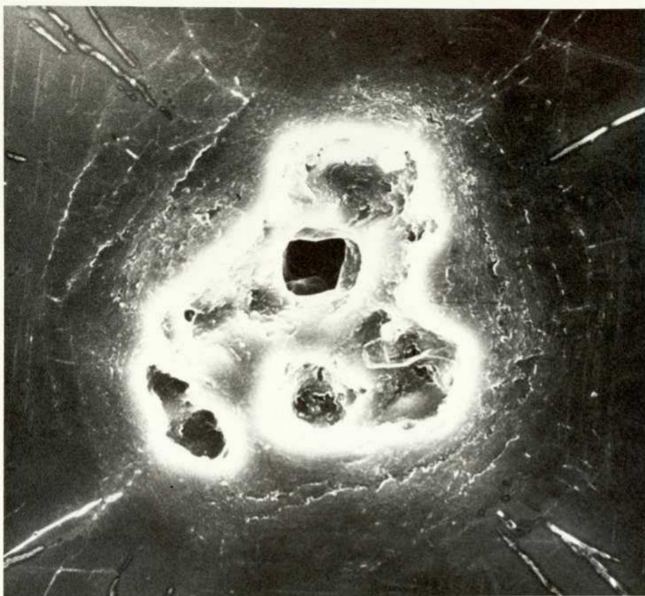
Fig 6.10 20ns Surface Damage in ADP ( \times 300 )
