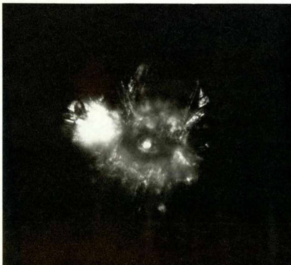
Fig 6-2(b) 20ns Inclusion Damage in ADP (x100)
