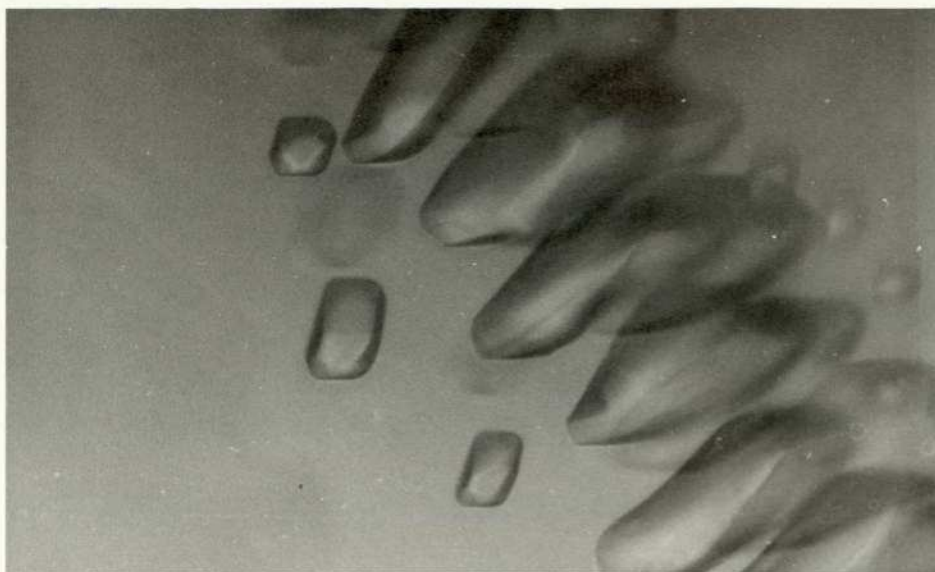
Fig 6.9(a) Growth Voids in KD*P( \times 200 )
