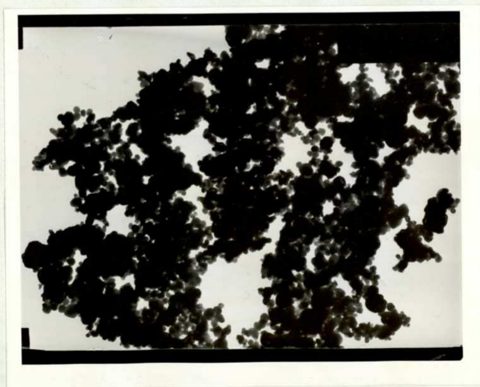
PLATE 3.2. NICKEL(II)OXIDE WITH 31 WEIGHT % LEAD(II)BROMIDE ( 10,000 x )
