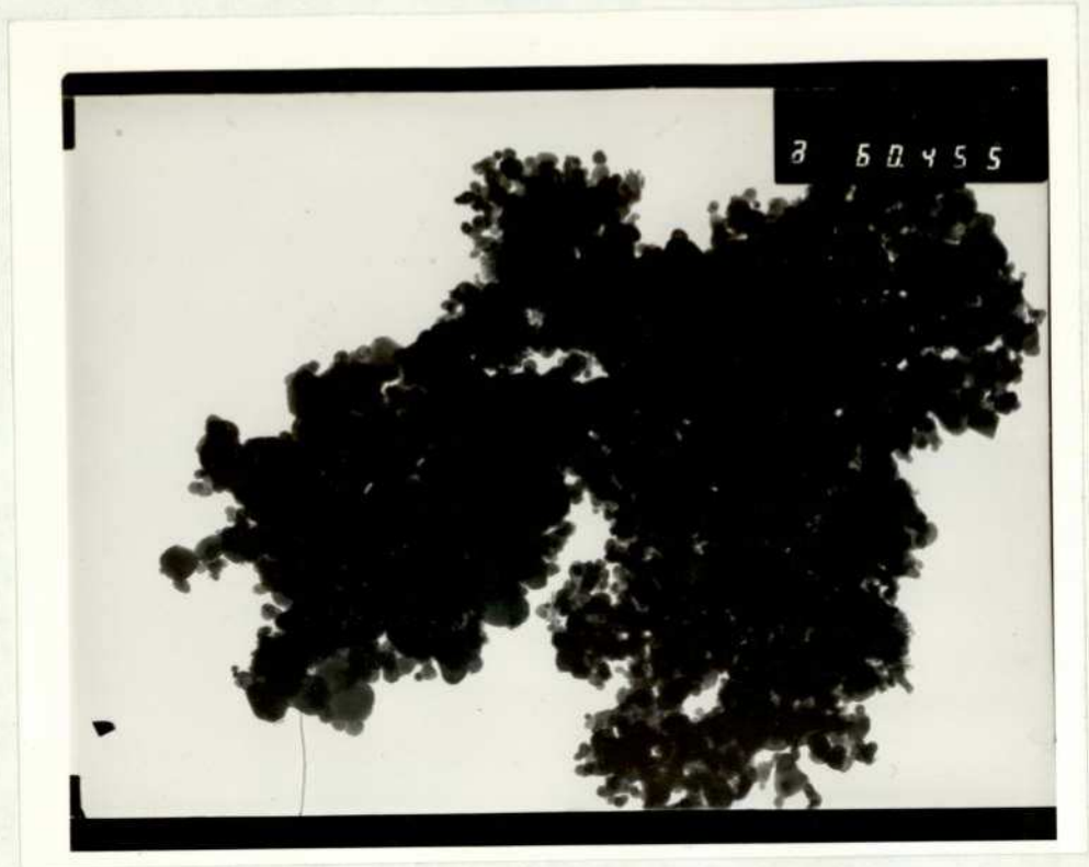
PLATE 3.13. ALUMINA SUPPORTED COBALT(II,III,III)OXIDE WITH 8.9 WEIGHT % LEAD(II)BROMIDE (20,000 x)
