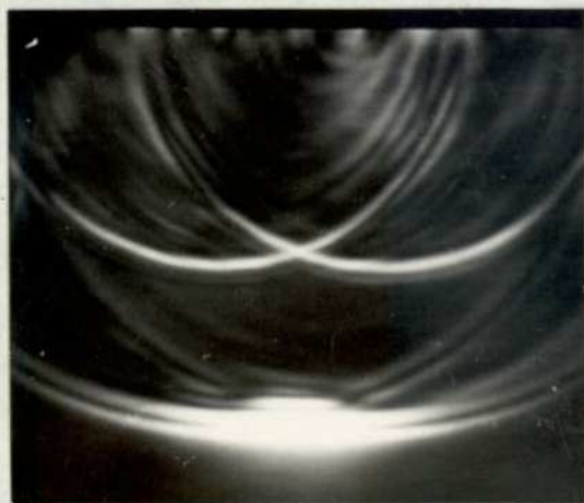
Fig.25 PHOTOELASTIC IMAGE OF THE PULSE STRUCTURE PRODUCED BY A COMPRESSION-WAVE TRANSDUCER (not seen) BONDED TO THE TOP SURFACE OF A GLASS BLOCK. (Acknowledgements to Dr.R.C.Wyatt).
