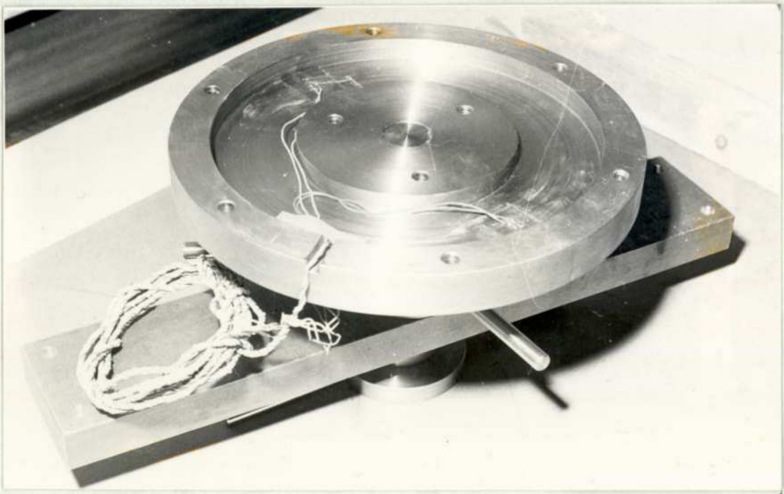
Fig.4.9 Load cell with the arrangement for altering 'entrefer'
