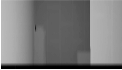
FIGURE 9 | The depth image extrapolated from the Velodyne 16-Line Puck sensor. [Color figure can be viewed at wileyonlinelibrary.com ]
