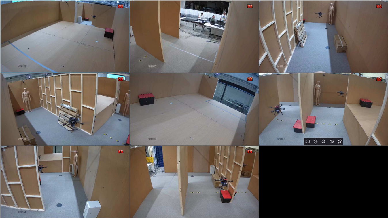
FIGURE 1 | The arena built for the Sapience competition as seen by the eight cameras used for monitoring the UAVs. [Color figure can be viewed at wileyonlinelibrary.com ]
