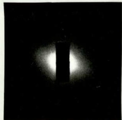
Fig. A1.3 Small-angle X-ray scattering from crab nerve bundles at various humidities; toroid optics
