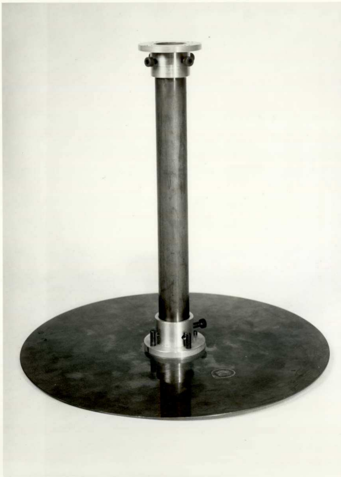
Tube and collar of the damping system
