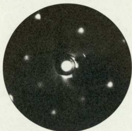
a) 43 V Pt(100) (2x2)-Cu/CO Adsorption at 20°C
