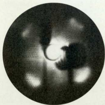
c) 122 V Diffuse pattern, as deposited
