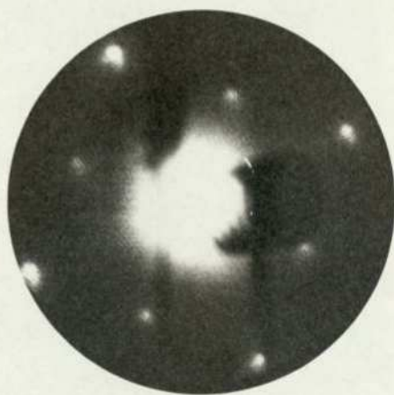
b) 55 V Pt(100) ( \sqrt{2} \times \sqrt{2} )R45°-Cu 9 M-L of Copper deposited on Pt(100) at 450°C
