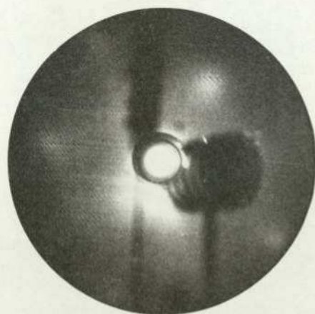
c) 34 V Pt(100) ( \sqrt{2} \times \sqrt{2} )R45°-Cu Oxygen on 9.3 M-L of Copper on Pt(100).
