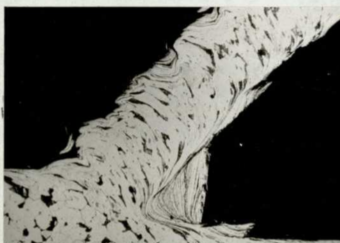
a. THREE PHASES OF CHIP FORMATION PHOTOMICROGRAPHS OF THE QUICKLY STOPPED CUTTING ACTION
