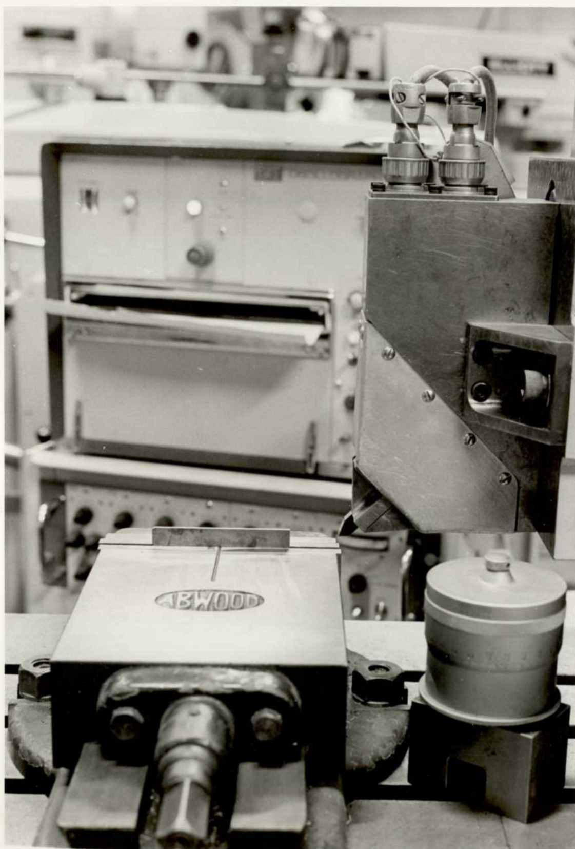
TWO COMPONENT DYNAMOMETER WITH INSTRUMENTATION & RECORDING EQUIPMENT
