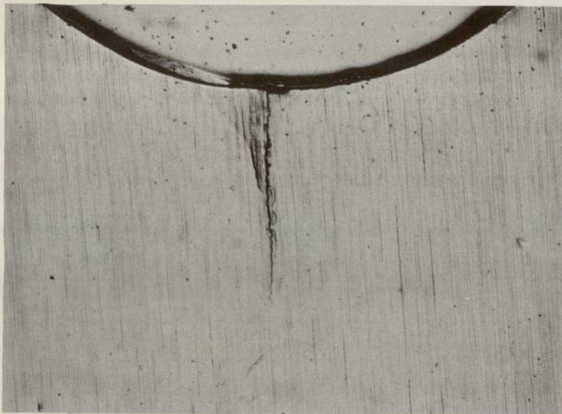
Fig.7 Crack of approximately 2 mm (approximate magnification: x27)
