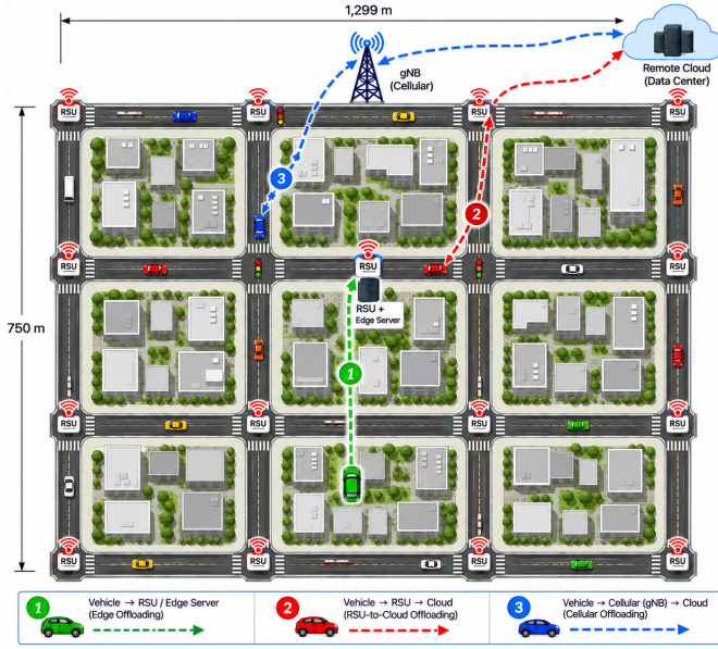
Fig. 1. Urban-grid vehicular edge-computing environment and the three execution paths implemented in the simulations: (1) vehicle \rightarrow RSU/edge server, (2) vehicle \rightarrow RSU \rightarrow cloud, and (3) vehicle \rightarrow cellular (LTE/5G) \rightarrow cloud. Edge compute is co-located with the RSU; vehicles generate tasks but local on-vehicle execution is not an orchestration action.
