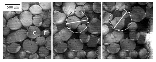
Figure 4. Deformation of globular Al-15Cu at  $^{\sim}70\%$  solid, highlighting the role of the rotation of an agglomerate of grains C and F with bowling pin shape. White dots mark the contacts important in causing rotation, white lines are the primary axis of the agglomerate formed by grains C and F, and the dashed line is the circle with diameter equal to the primary axis of the agglomerate. The push plate can be seen to the far right of each image.
