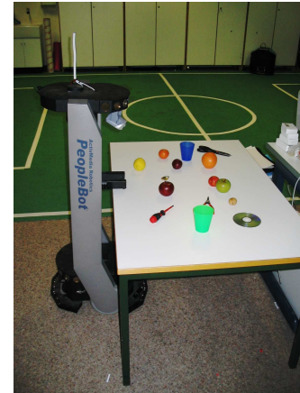
Figure 1. The robot standing in front of a white table. Different objects are laying on the table. The robot has to grasp or point to objects specified in simple command sentences.
