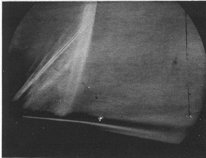
Vane Vortex Generators (Attached Flow)
