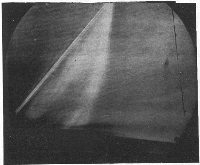
Figure 5.49 Experimental Pressure Distributions with Corresponding Schlieren Image for the 10% Bump with Small Air Jets ( $P_b/P_0=1.6$ )
