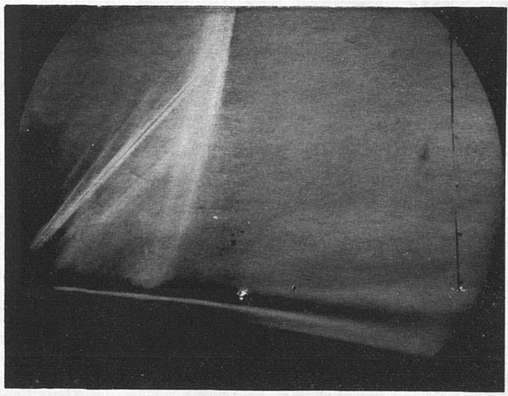
Figure 6.10 Experimental Pressure Distribution with Corresponding Schlieren Image for the 10% Bump with Vane Vortex Generators.
