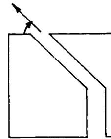
Jet Inclination:  $\theta=45^\circ$
