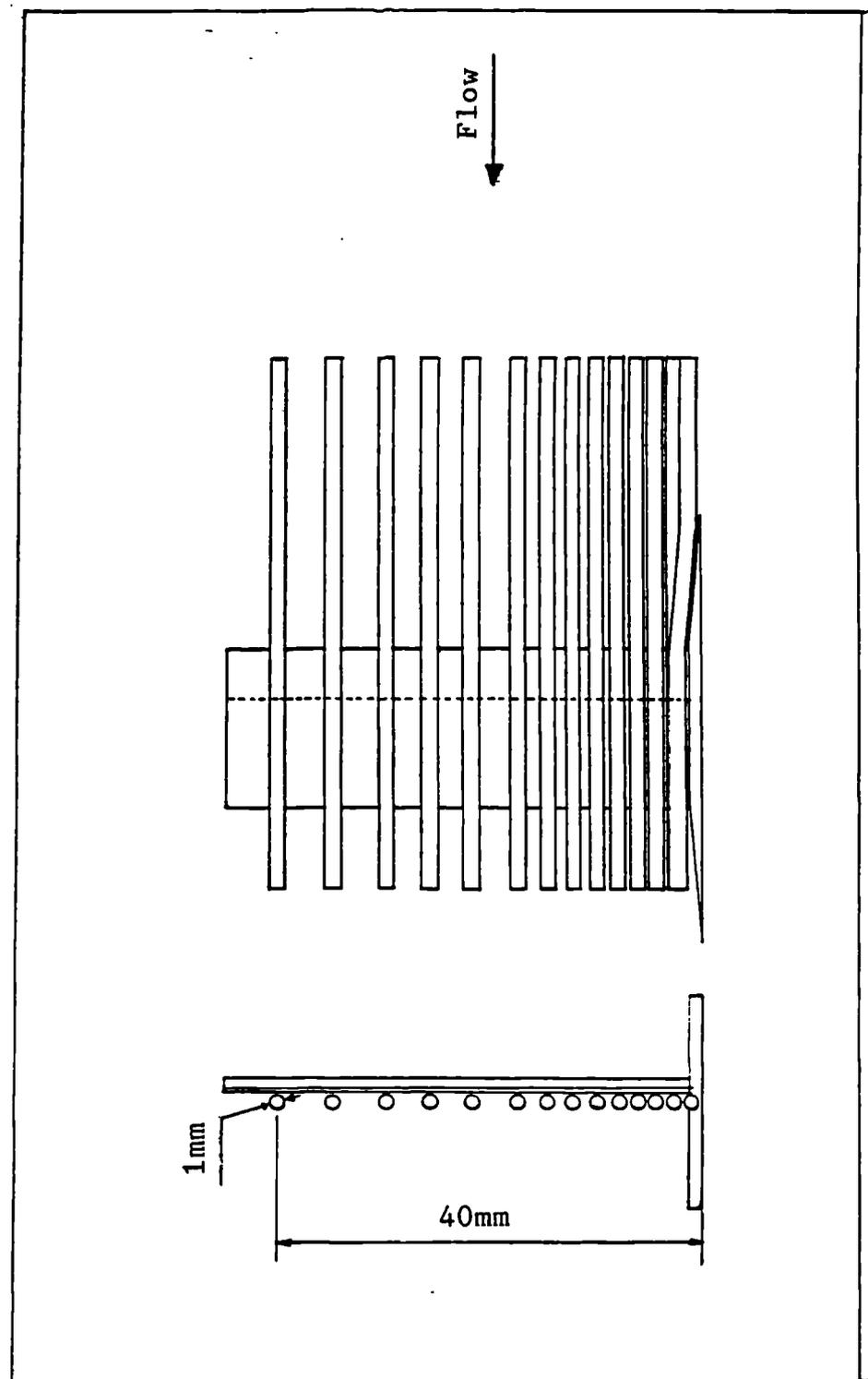
Figure 3.12 Diagrammatic Representation of the Boundary Layer Rake
