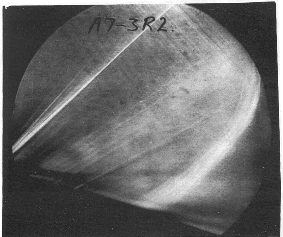
Figure 5.66 Experimental Pressure Distributions with Corresponding Schlieren Image for the 14% Bump with Large Air Jets ( $\theta=60^\circ$ ,  $P_b/P_0=1.5$ ).
