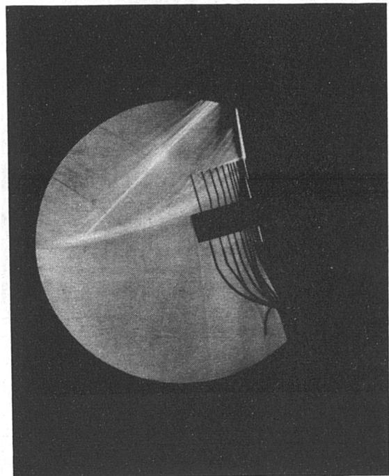
Figure 5.75 Boundary Layer Profiles With Vane Vortex Generators.
