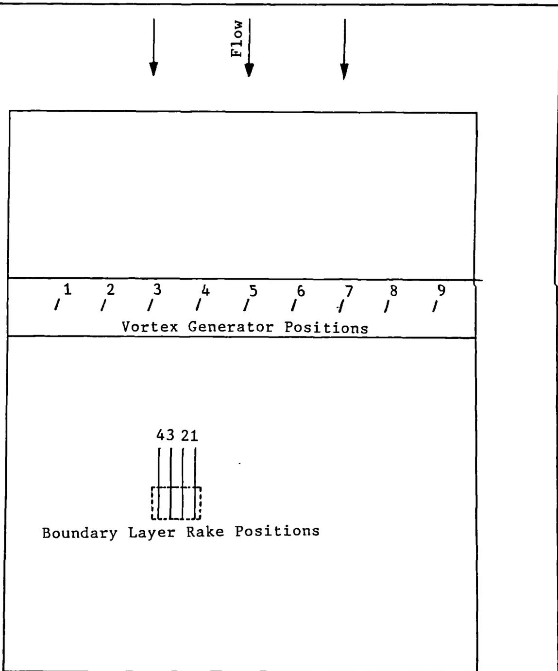
Figure 3.13 Model Arrangement for Boundary Layer Rake Investigation
