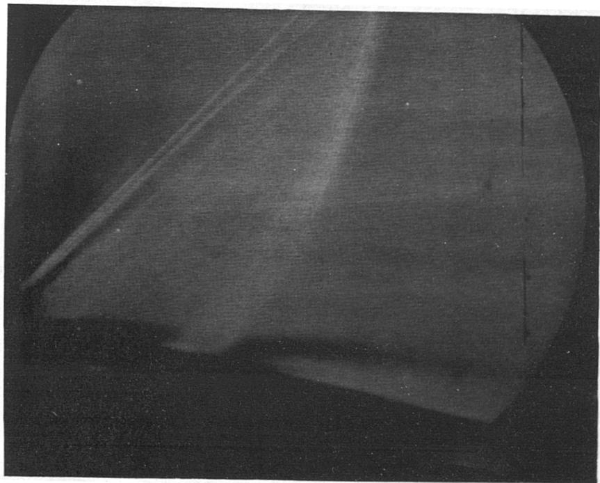
Figure 5.59 Experimental Pressure Distributions with Corresponding Schlieren Image for the 10% Bump with Large Air Jets ( $\theta=60^\circ, P_b/P_0=1.2$ ).
