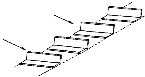
Figure 1.1 Vane Vortex Generators
