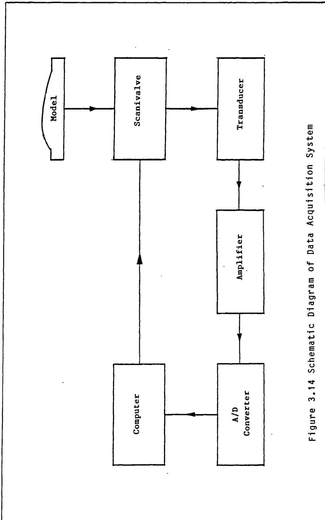
Figure 3.14 Schematic Diagram of Data Acquisition System
