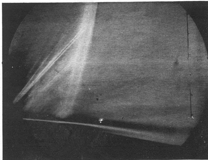
Figure 5.43 Experimental Pressure Distribution with Corresponding Schlieren Image for the 10% Bump with Vane Vortex Generators.
