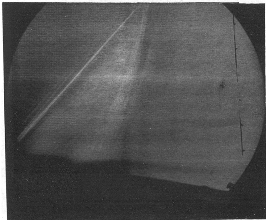
Figure 5.47 Experimental Pressure Distributions with Corresponding Schlieren Image for the 10% Bump with Small Air Jets ( $P_b/P_0=1.2$ )
