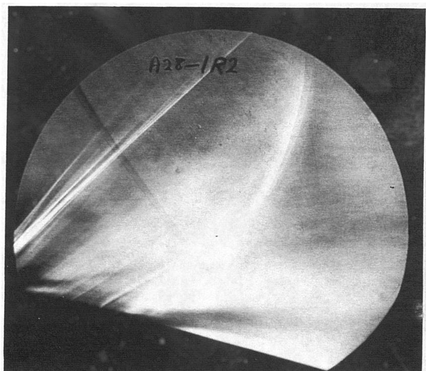
Figure 5.54 Experimental Pressure Distributions with Corresponding Schlieren Image for the 14% Bump with Small Air Jets ( $\theta=30^\circ$ ,  $P_b/P_0=1.6$ ).
