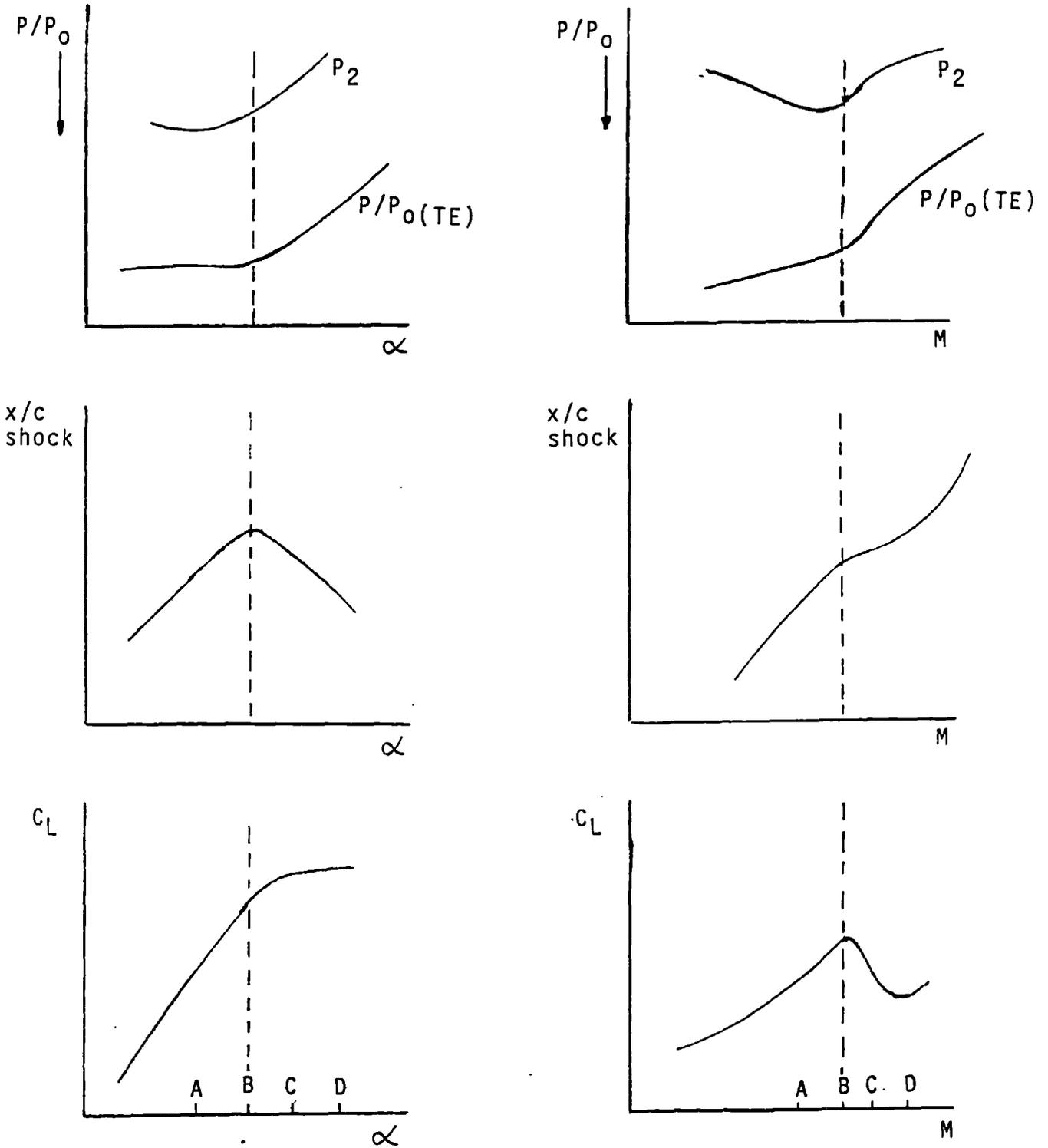
Figure 2.3 Comparison of Aerofoil Characteristics
