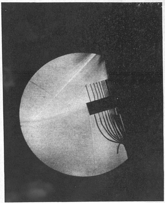
Figure 5.79 Boundary Layer Profiles With Small Air Jet Vortex Generators
