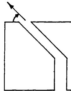
Jet Inclination:  $\theta=45^\circ$
