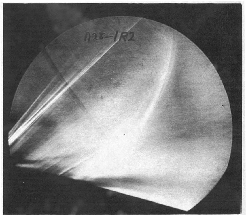
Figure 6.19 Experimental Pressure Distributions with Corresponding Schlieren Image for the 14% Bump with Small Air Jets ( $\theta=30^\circ$ ,  $P_b/P_0=1.6$ ).
