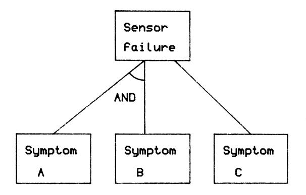
Fig.6.3 Diagnosis of sensor failures
