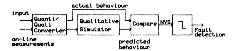
Fig.6.1 Fault detection
