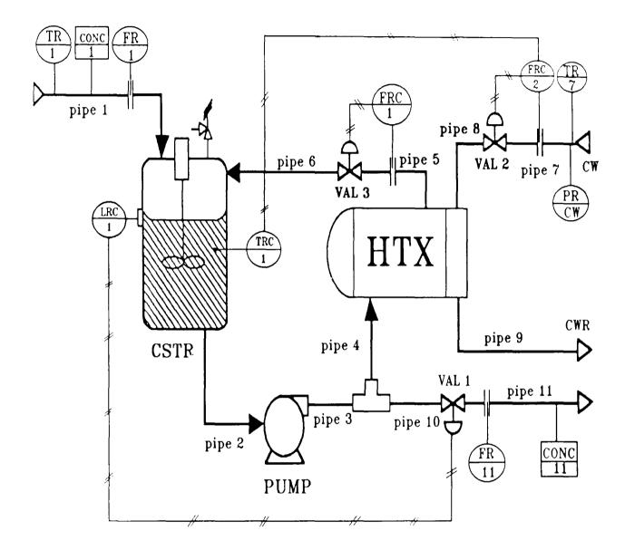
Fig.4.7 Continuous stirred tank reactor with recycle
