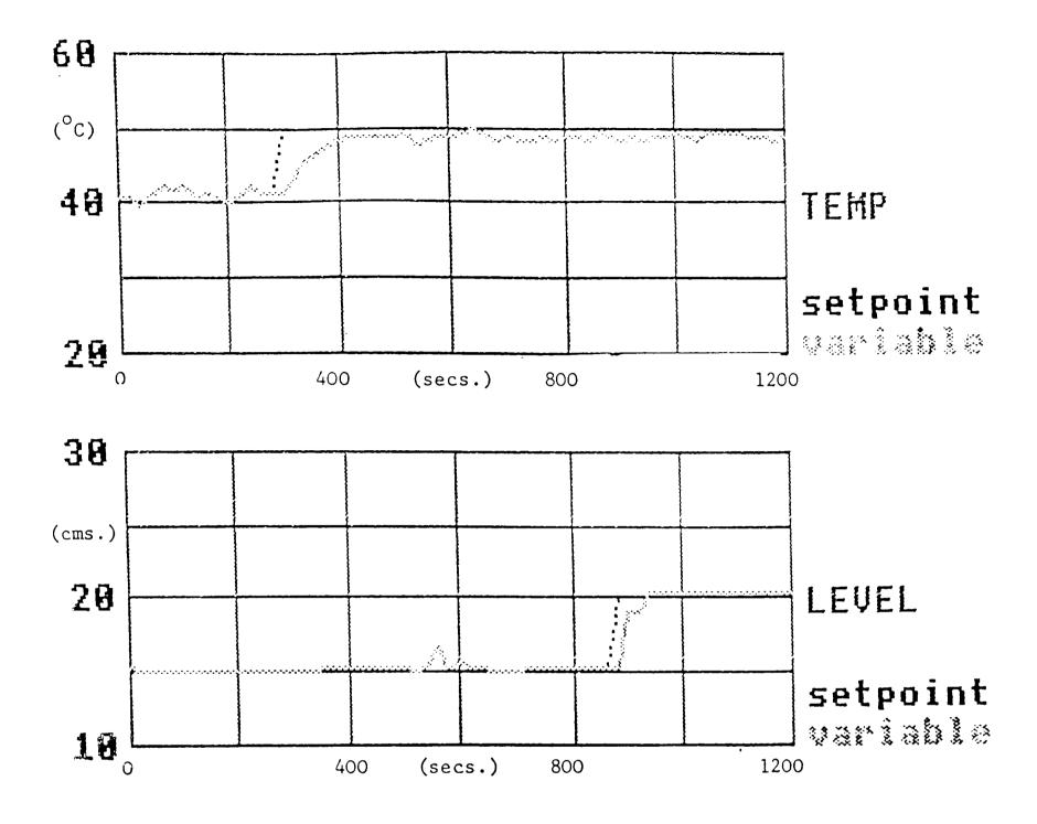
Figure 3.2 Response of the rule based controller
