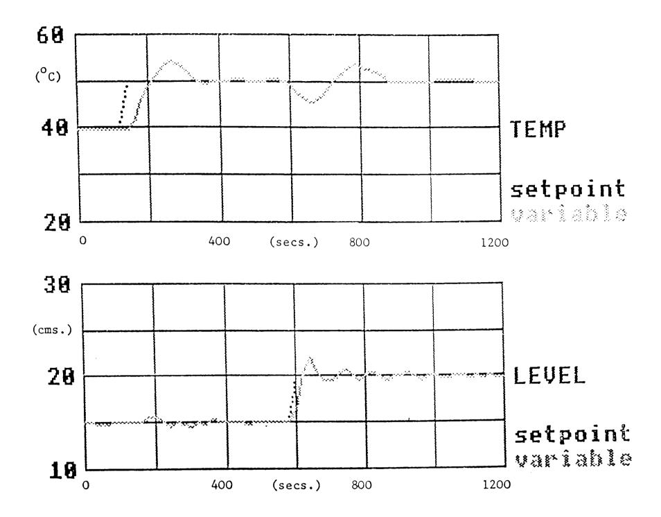
Figure 3.3 Response of the decoupling PI controller
