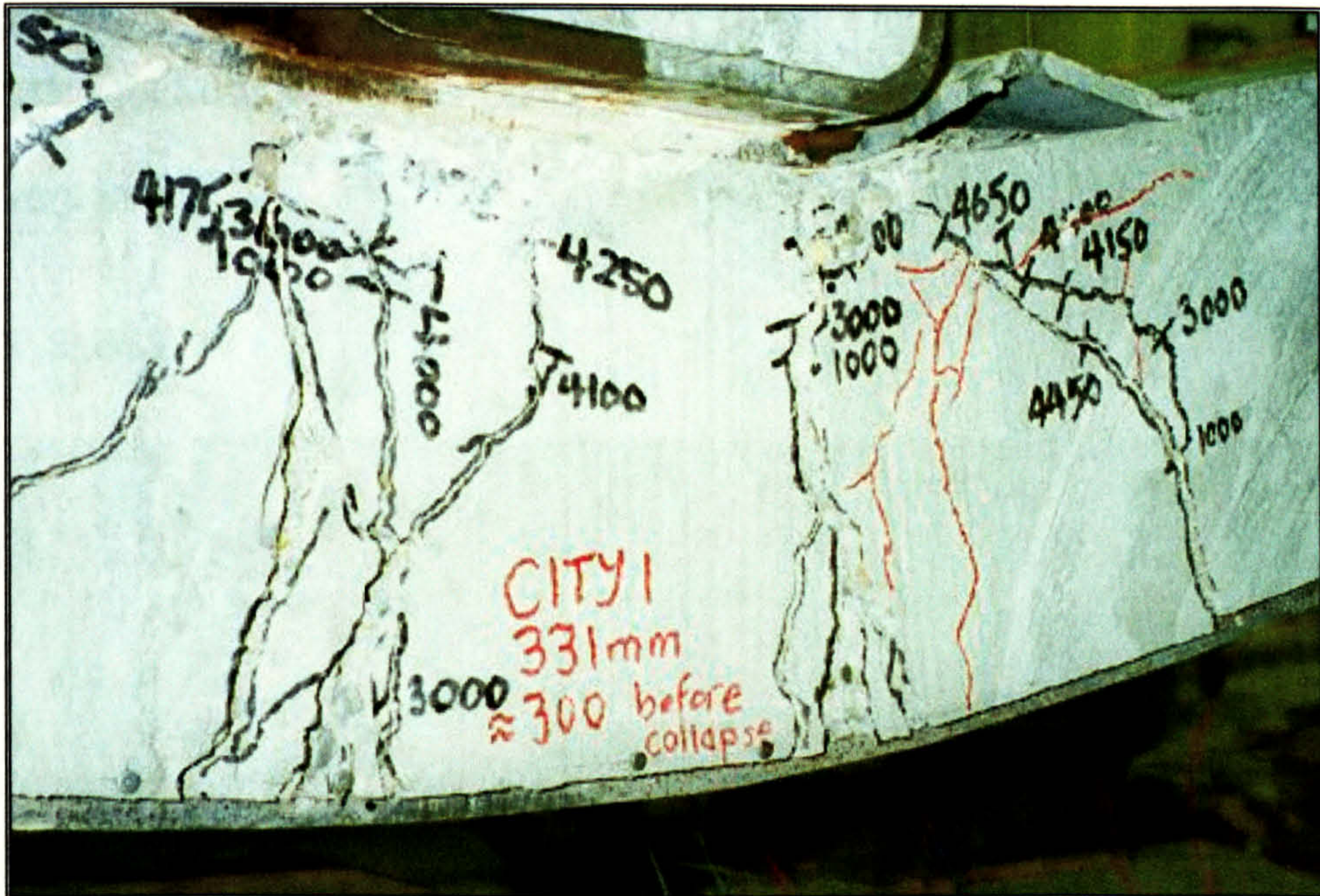
Plate 3.2. City1 crack patterns.
