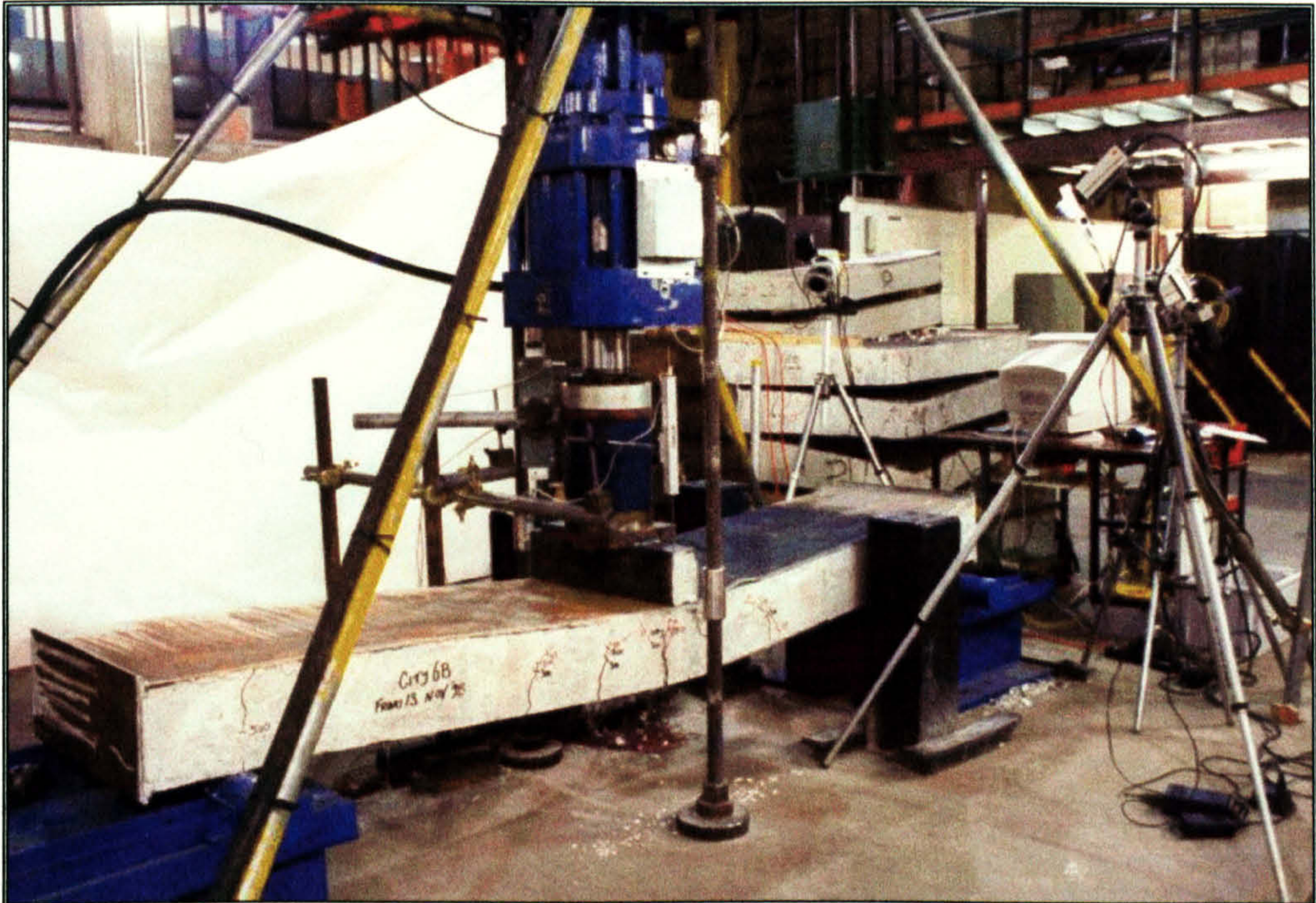
Plate 3.5 Overall set up using CCD cameras.
