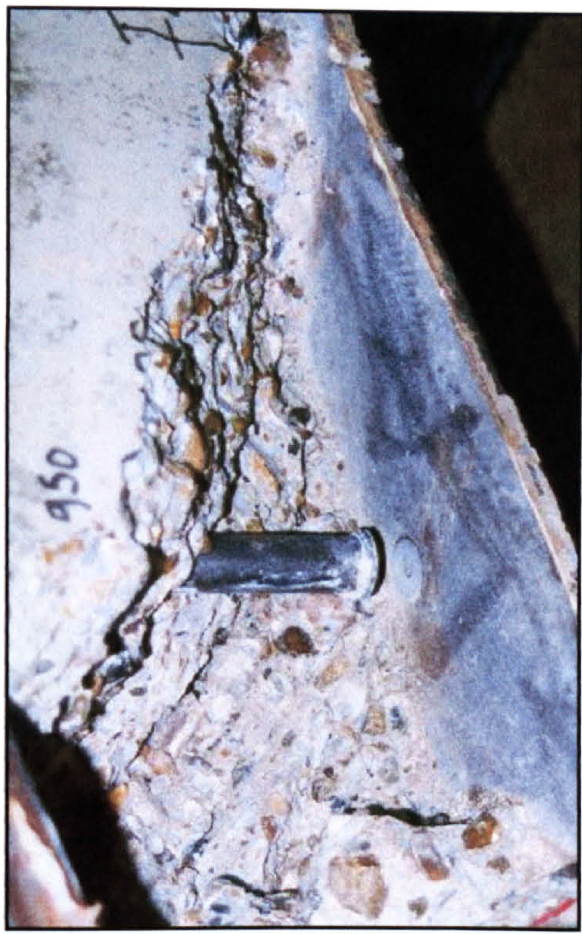
Plate B4c. Close-up of failed area showing connector weld failure.
