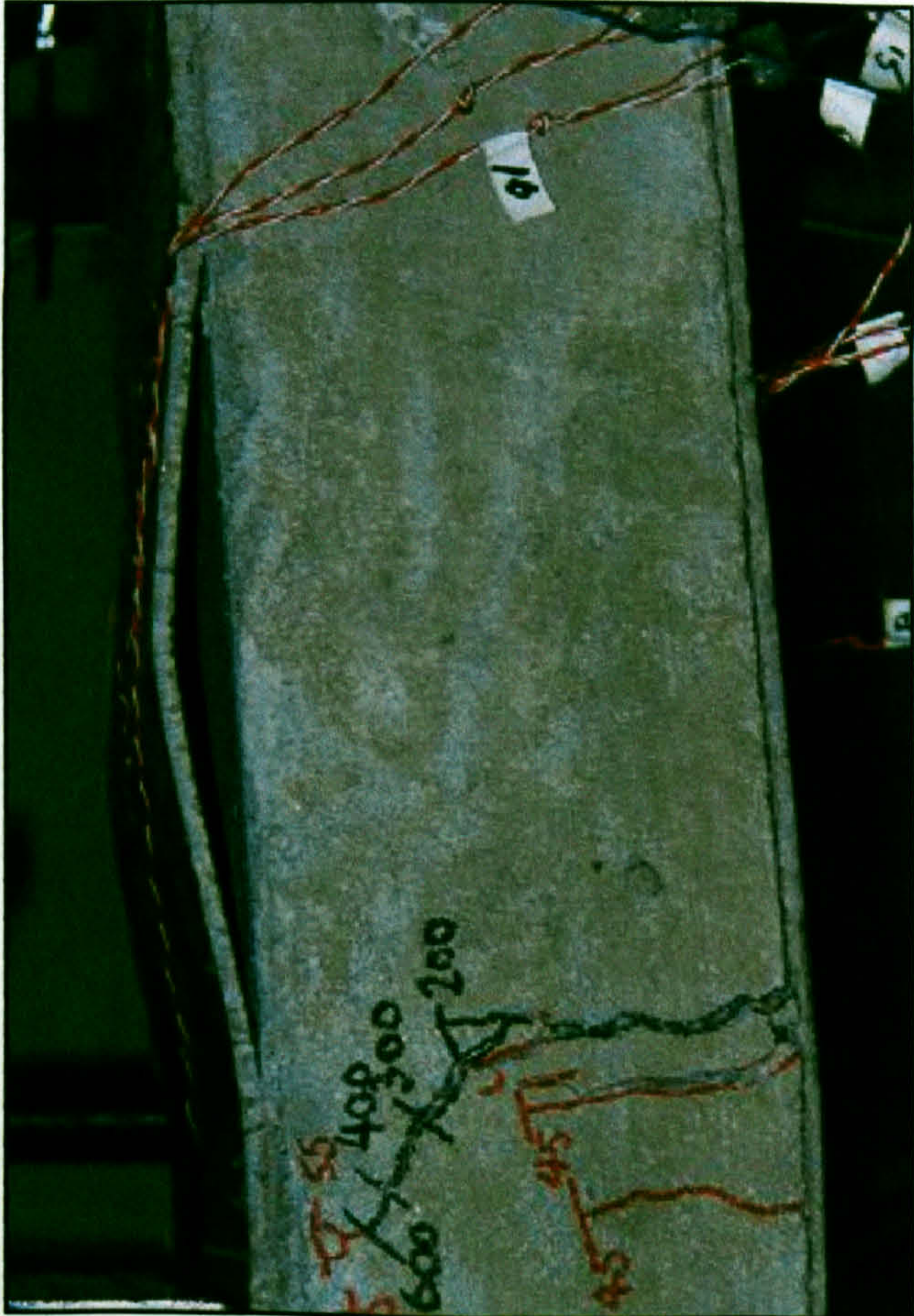
Plate B13b. Close-up of failed area showing local buckling and lack of cracking to the right of the picture, where another shear connector is located.
