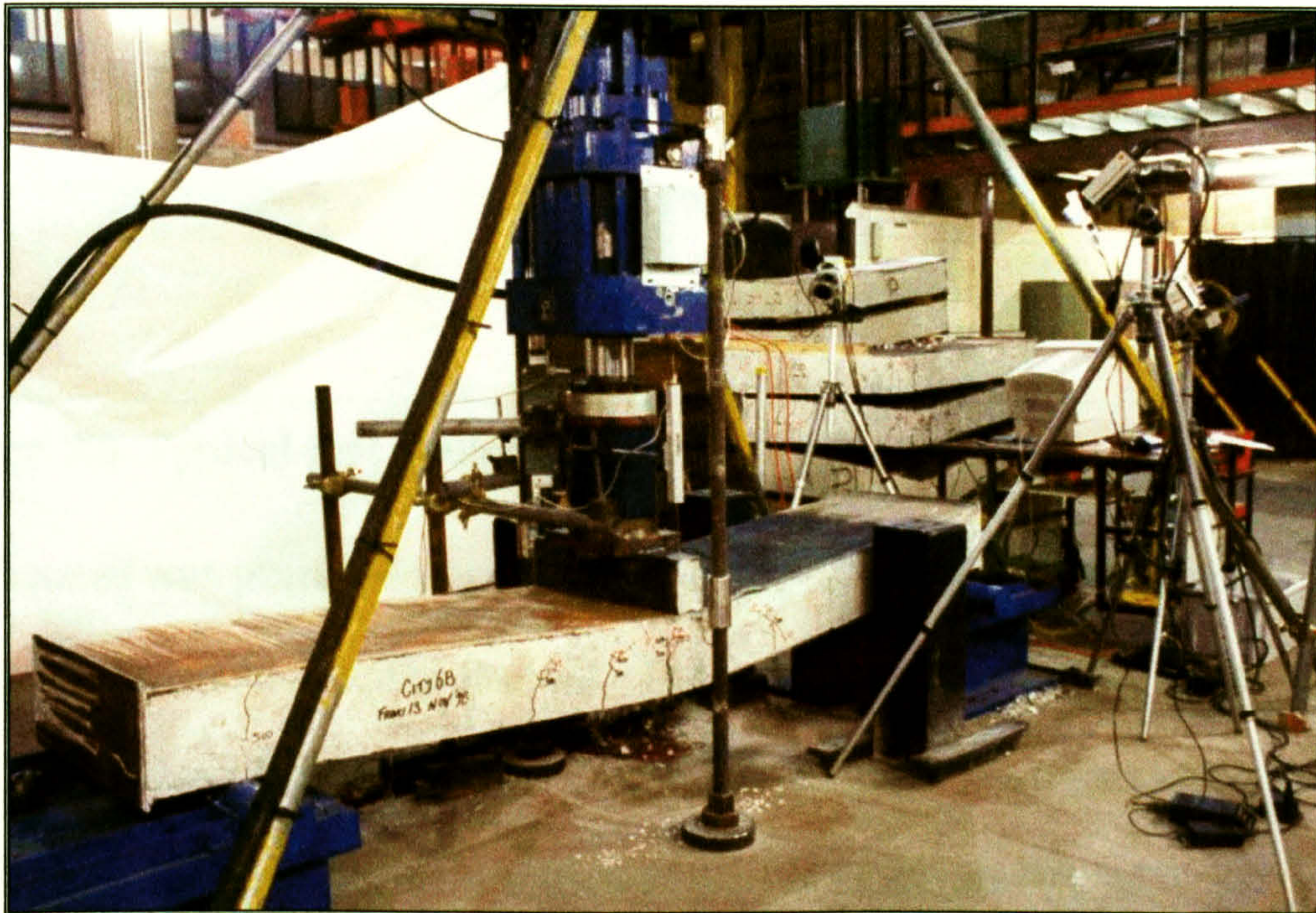
Plate 3.1. Test Rig with 1000kN Actuator
