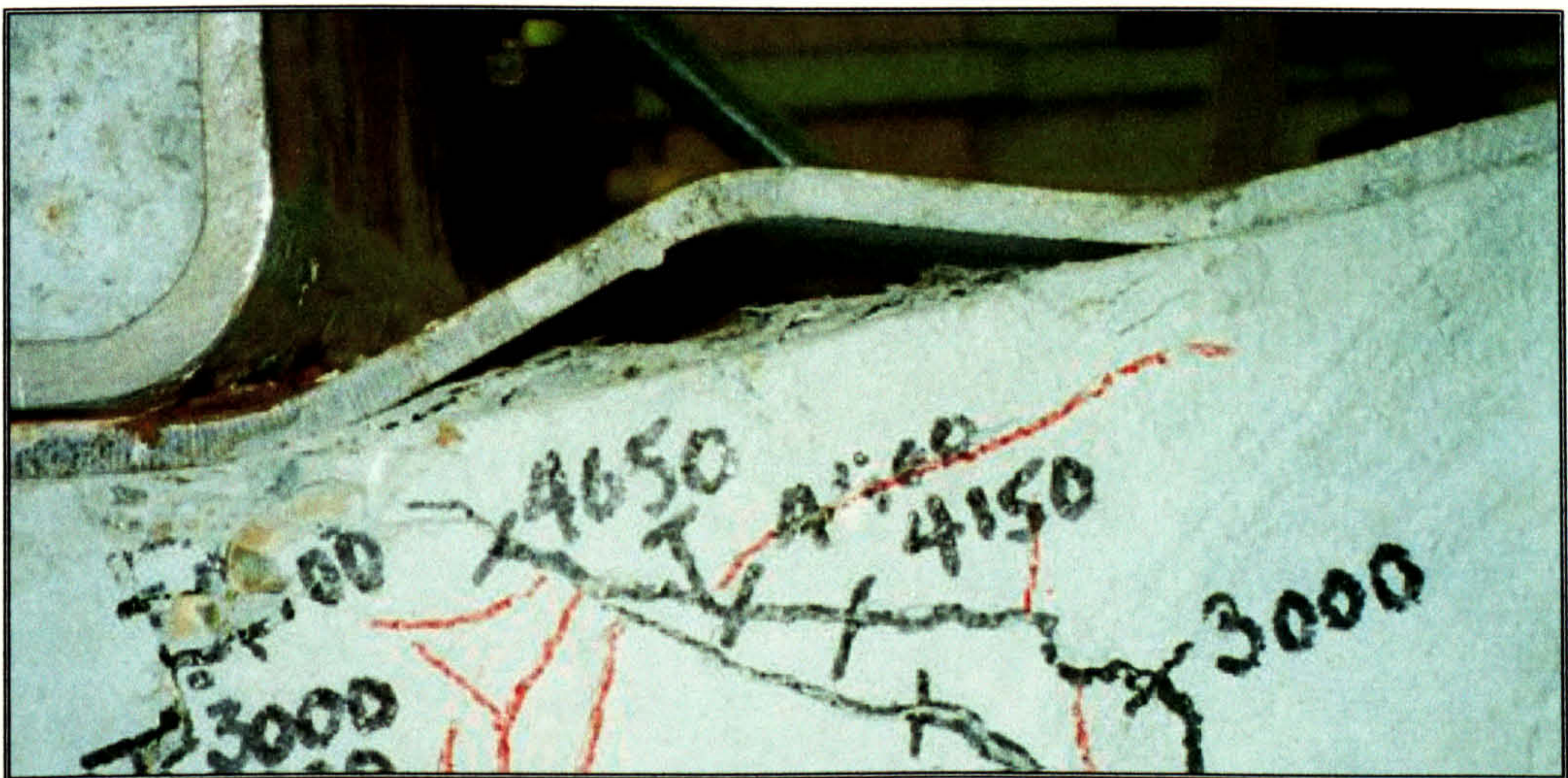
Plate 4.3. Buckling of Compression plate of City1
