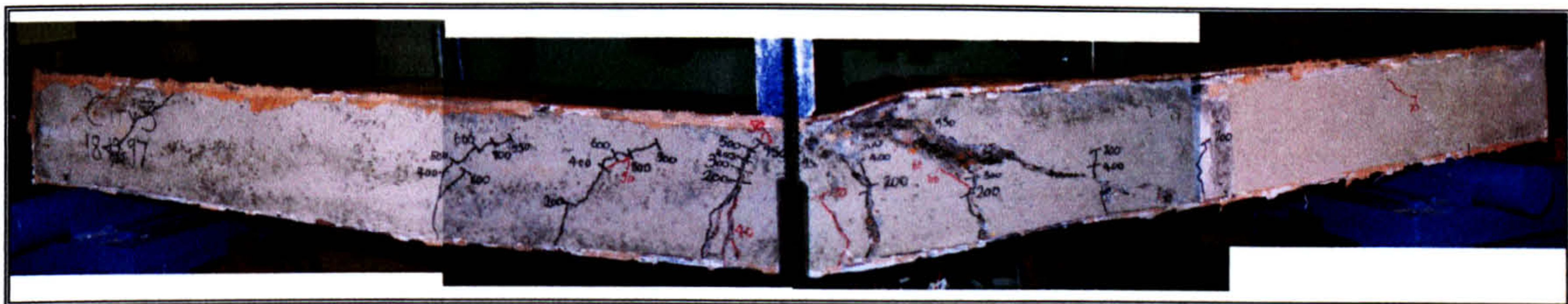
Plate 3.7. City3 crack patterns.
