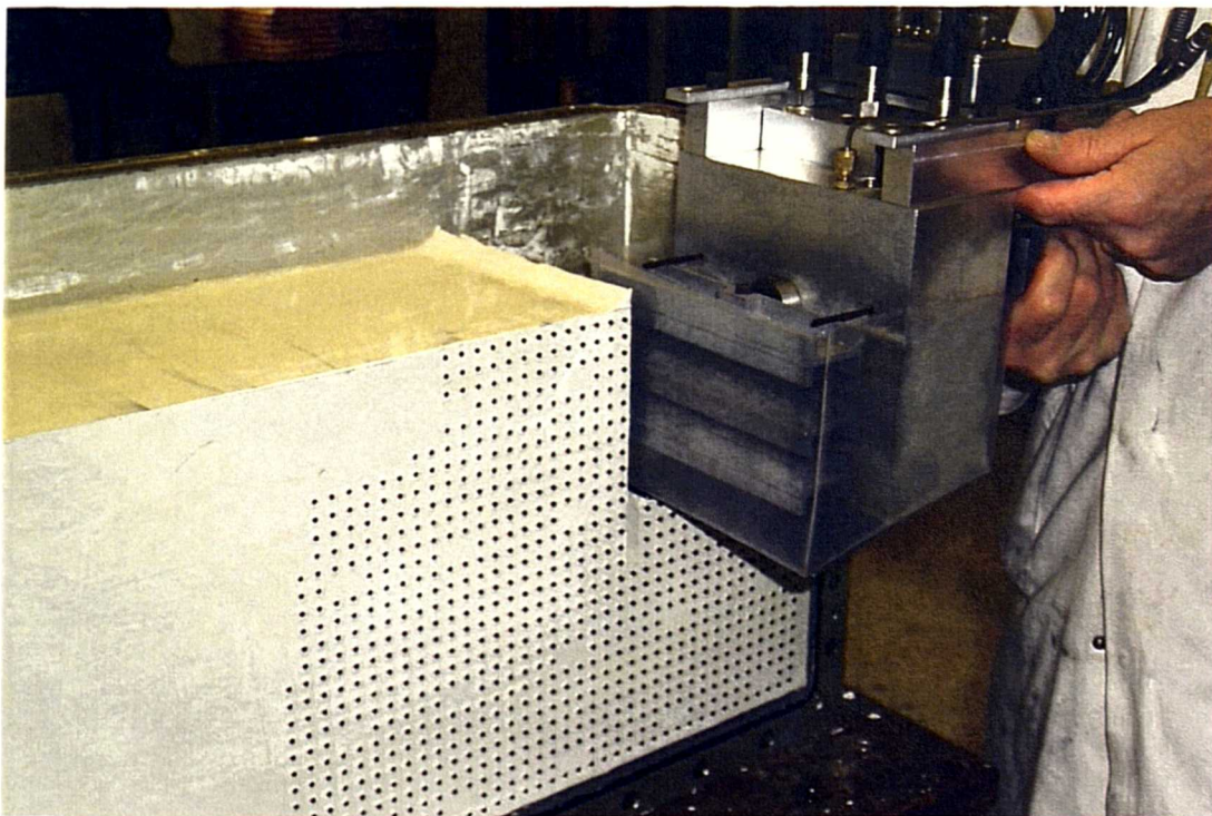
Figure 3.43 Installing prop module apparatus into the strongbox
