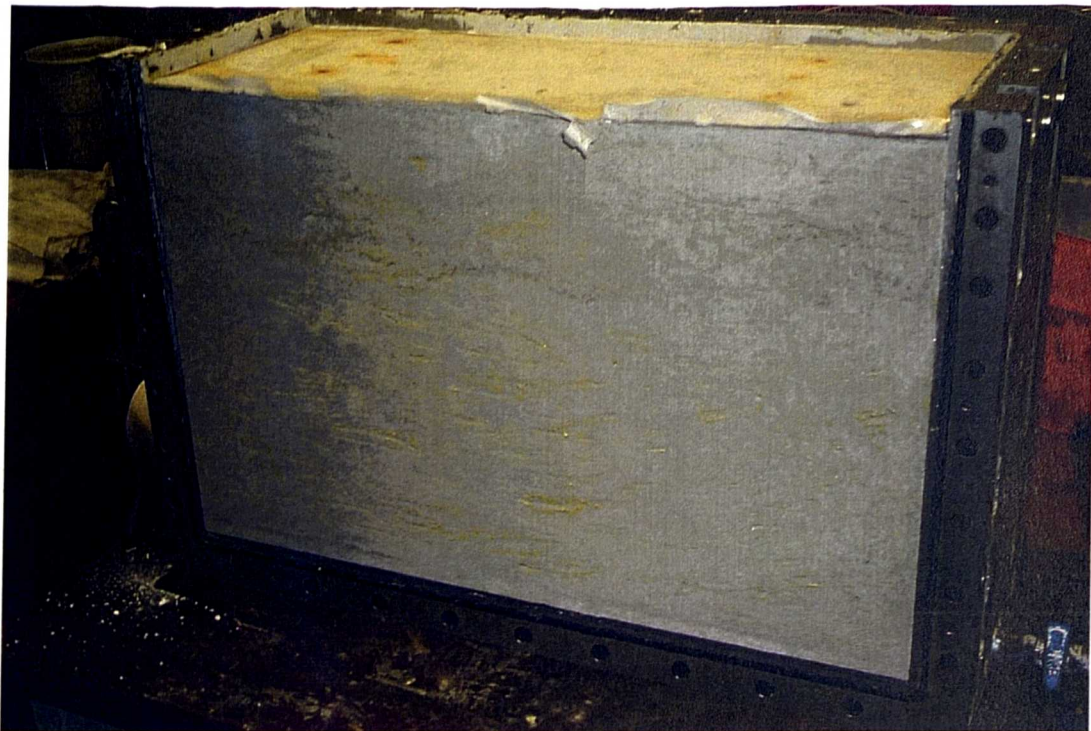
Figure 3.30 A typical soil sample immediately after removal from the consolidation press. Excess water pump grease that accumulated on the front surface was carefully scraped off to enable good contrast for image processing
