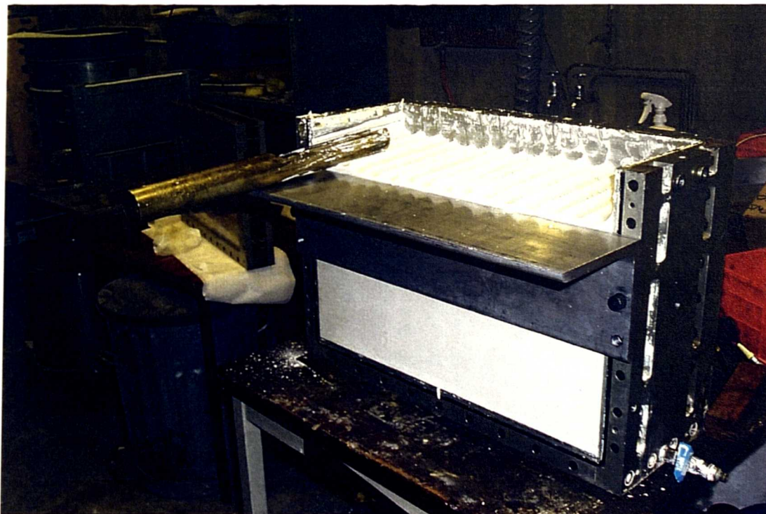
Figure 3.31 Top surface of the sample was trimmed to the approximate level using a 50mm diameter brass tube cutter
