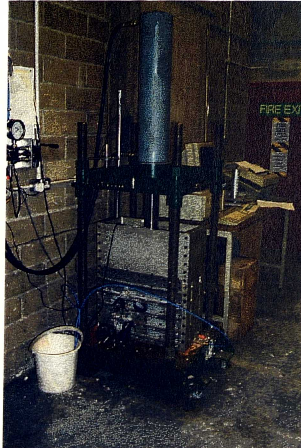
Figure 3.28 Consolidation press used for sample preparation prior to model making
