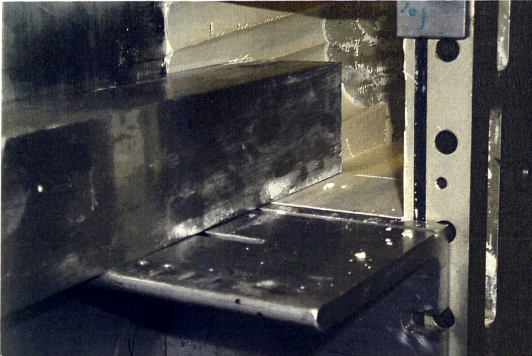
Figure 3.36 Trimming of excavation using aluminium box section cutter
