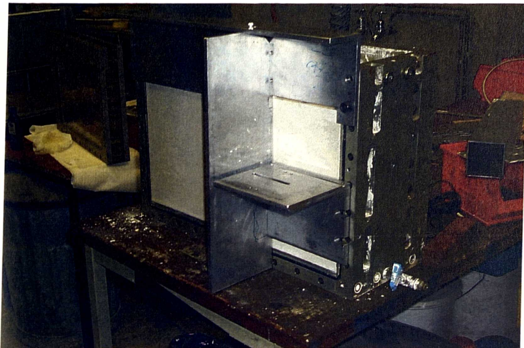
Figure 3.34 Jig used for forming excavation and trench for embedded wall
