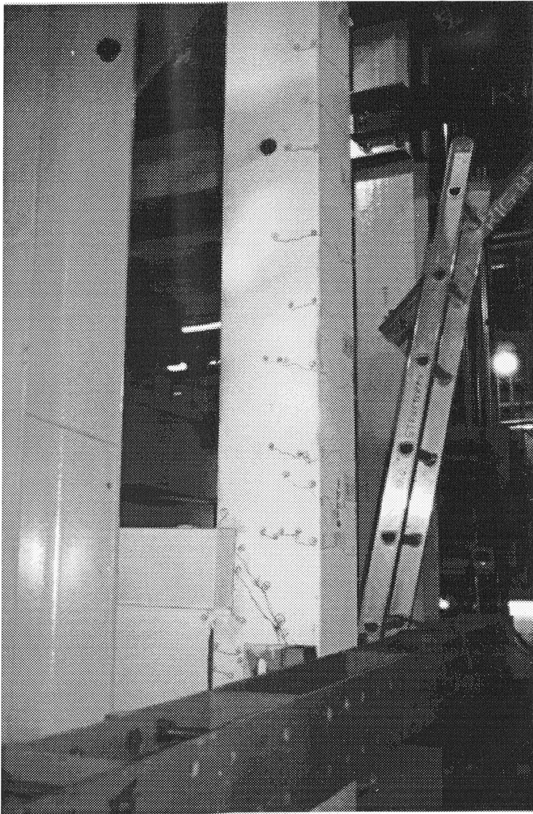
FIG.4.18 CRACK PATTERN IN THE UPPER COLUMN
