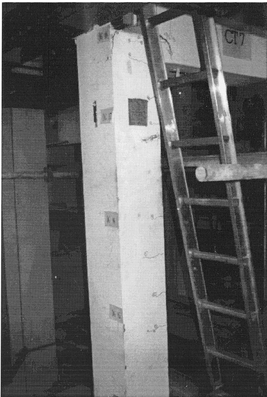
FIG.4.19 CRACK PATTERN IN THE LOWER COLUMN
