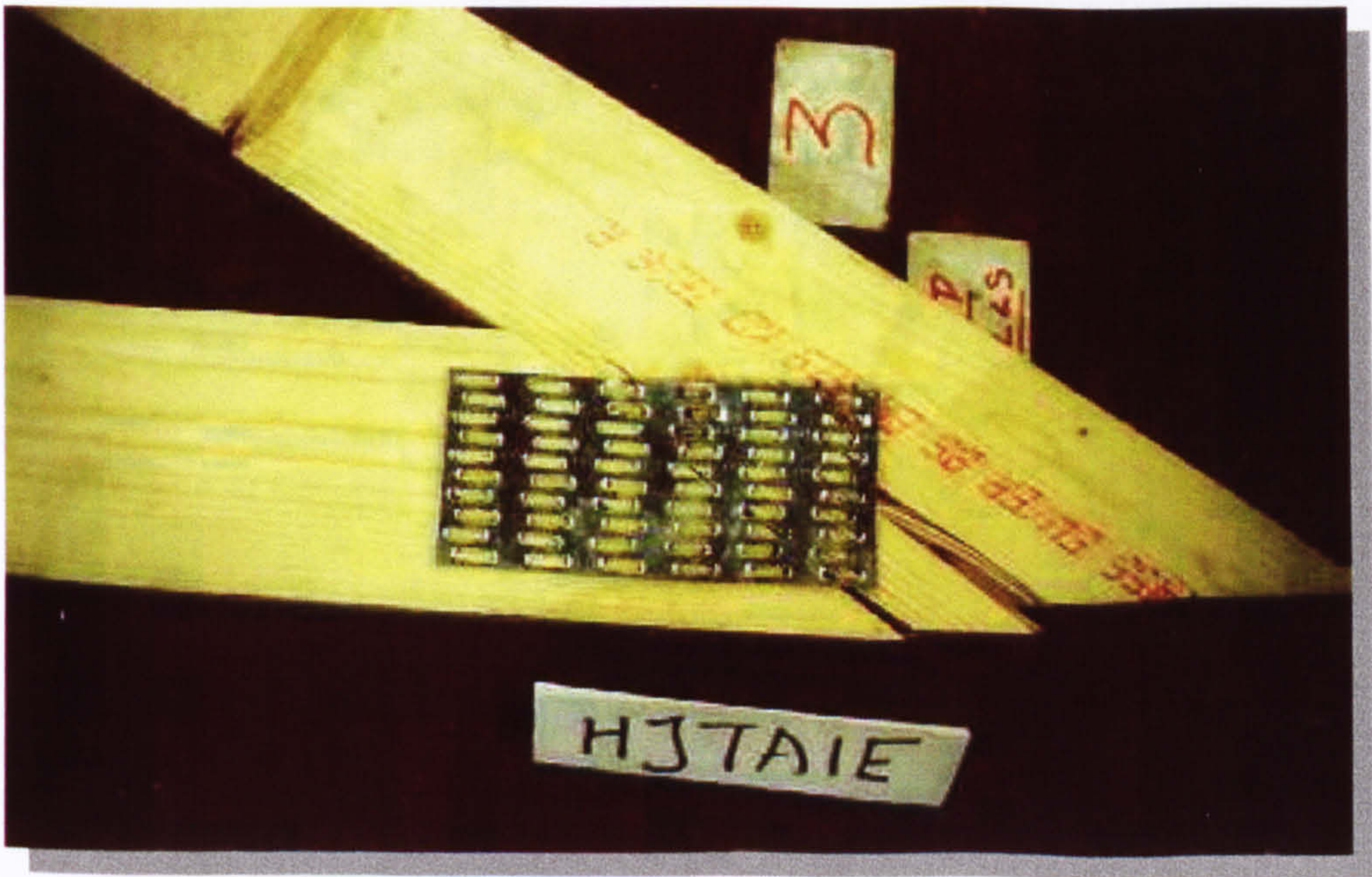
Fig. 6.3.3 – Failure mechanism for HJTA series test
