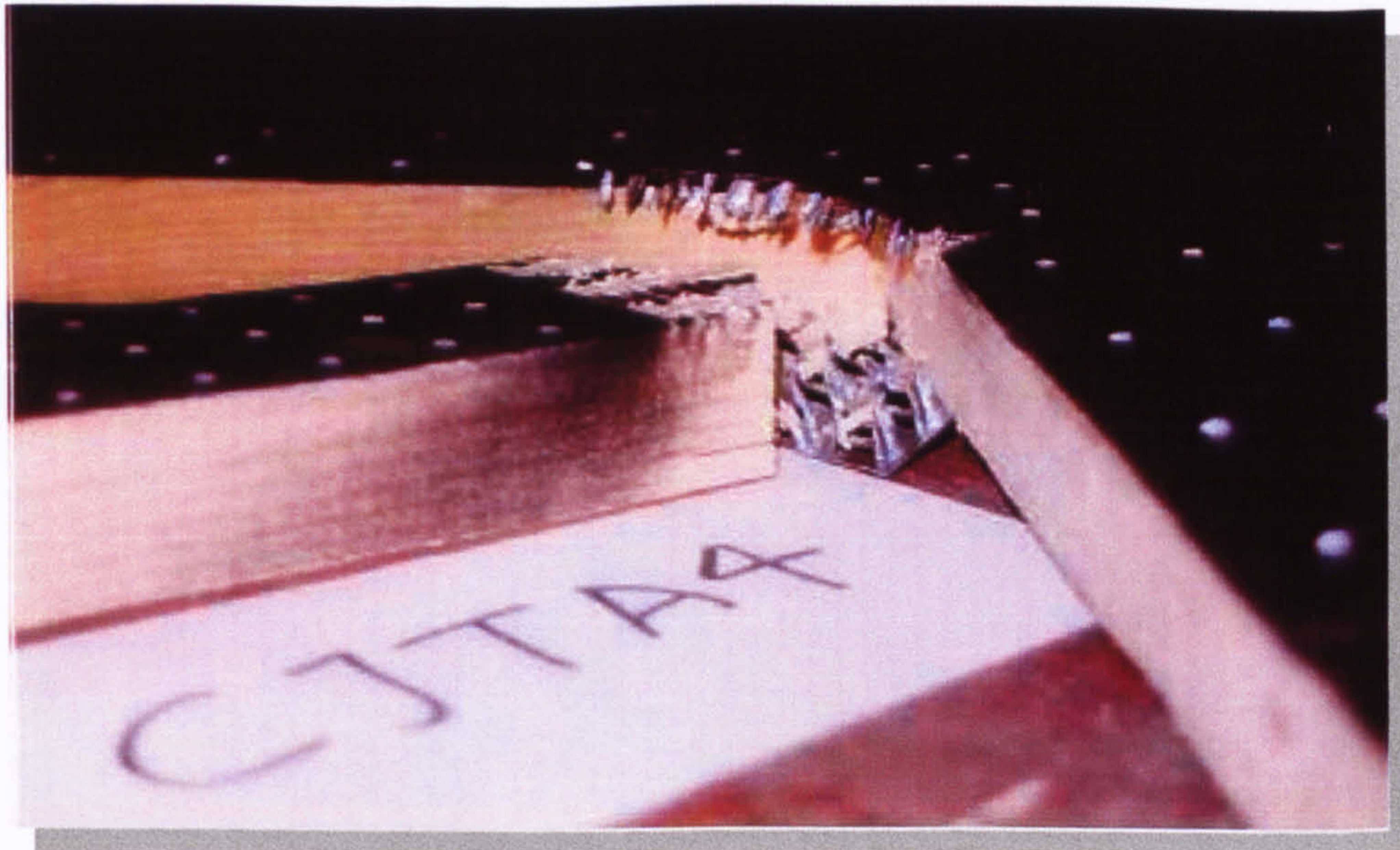
Fig. 6.2.3 – Bending moment load failure
