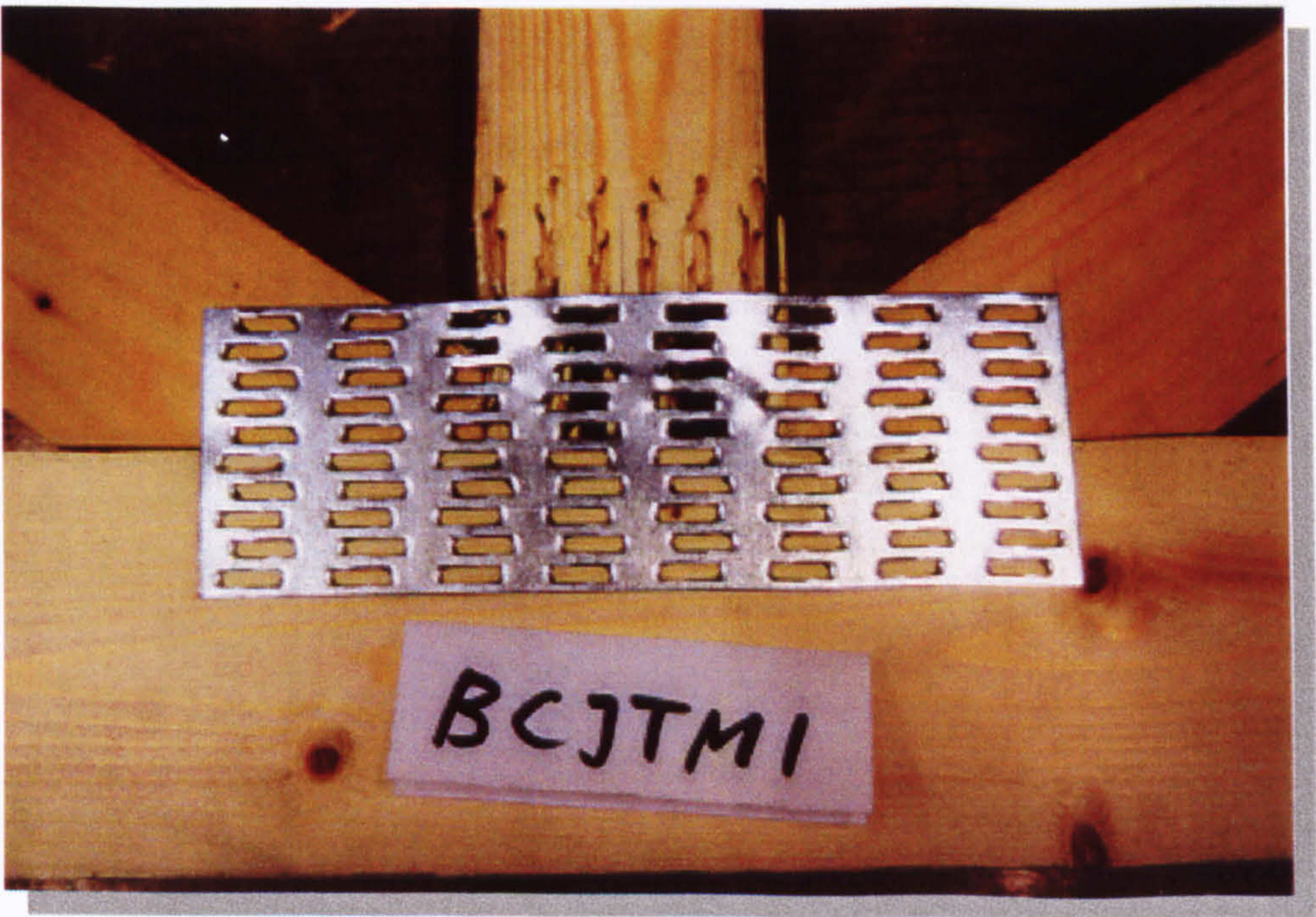
Fig. 6.5.1 – Typical failure of BCJTM test series
