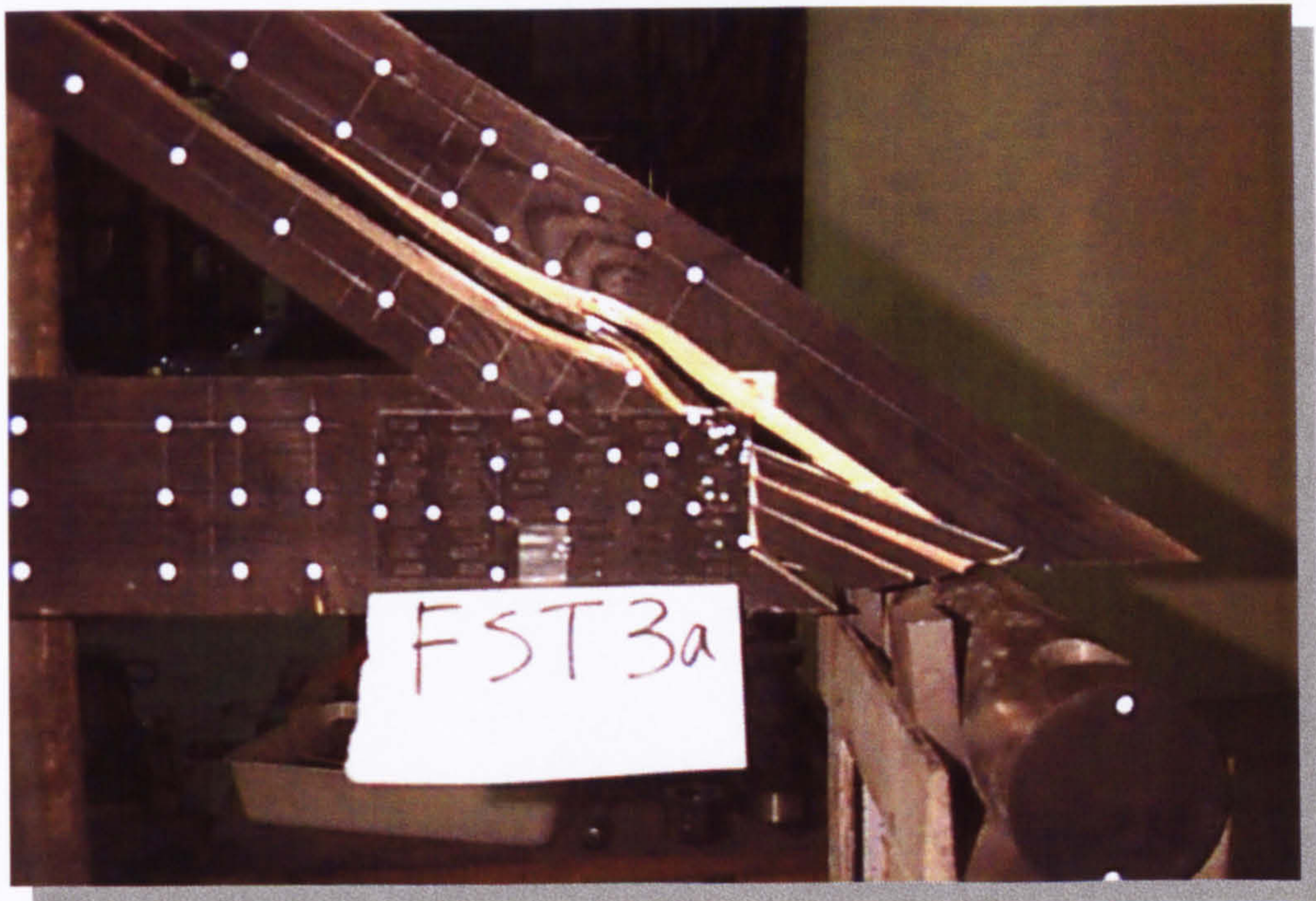
Fig. 6.7.2 – Failure mode for support at the rafter for test FST3
