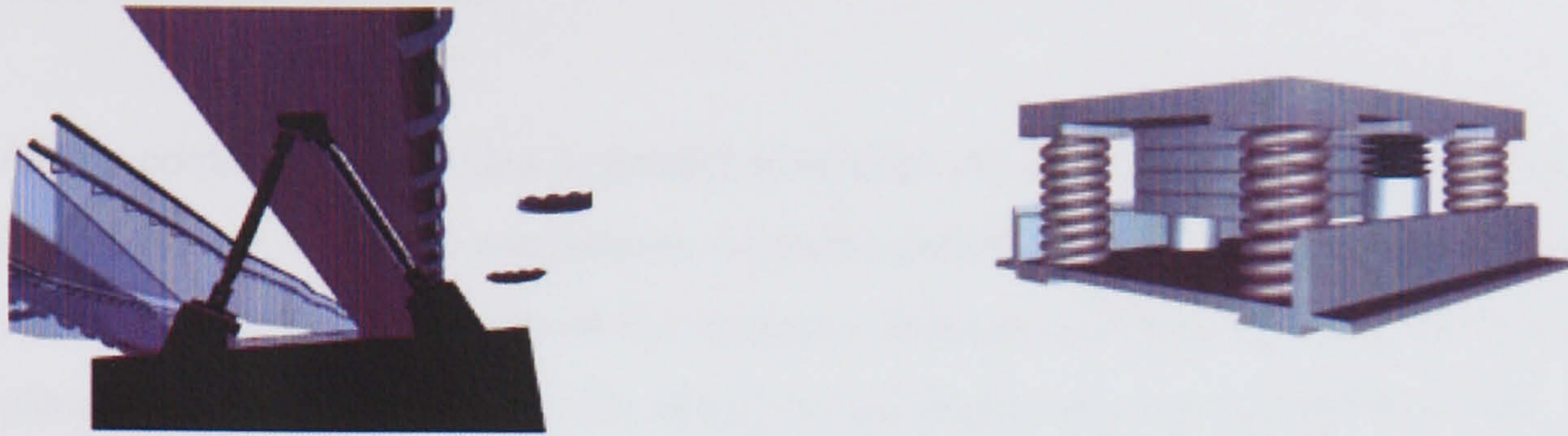
Figure 2.9. Dampers on millennium bridge Source: [Arup n.d.]
