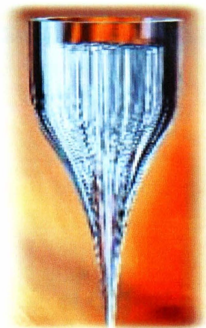
Fig. 2.5: Array of hollow capillary silica tubes bundled around a pure silica rod replacing the centre capillary [Kristiansen].
